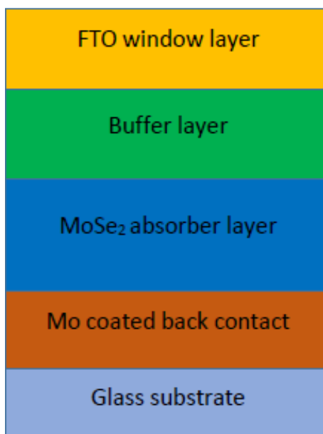
Fig. 1. Schematic diagram of MoSe 2 solar cell.
