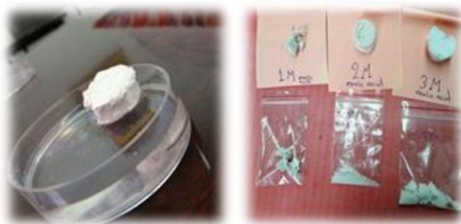
Fig. 4. The last shape of the silica aerogel prepared and the floating property.
