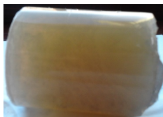
Fig. 1. Agarose gel phantom with ferrite nanoparticles.
