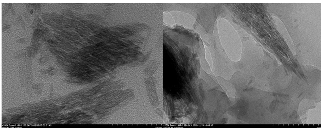
Fig. 4. (a) TEM image of CS-DB15, (b) CS-DB15 after bionano-fenton reaction
