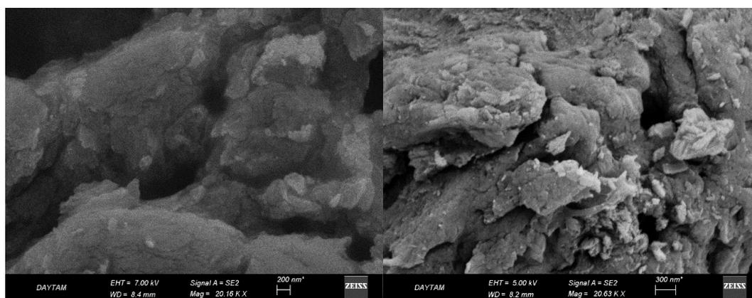
Fig. 5. (a) SEM image of CS-DB15, (b) CS-DB15 after bionano-fenton reaction
