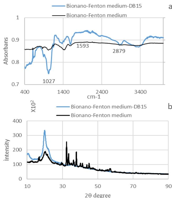
Fig. 3. (a) FT-IR spectra of adsorbents 3(b) XRD spectra of adsorbents
