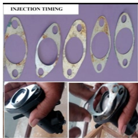
Fig. 1. Fuel injection parameters modifications.
