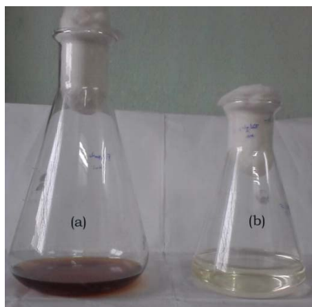
Fig.-1 the change of color from light yellow (b) to light brown (a) of live cell filtrate (LCF) of Aspergillus foetidus after addition of \text{AgNO}_3 solution (1 mM).
