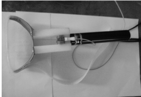
Fig. 3. The Support Attachment and the needle attachment connected to the linear actuator
