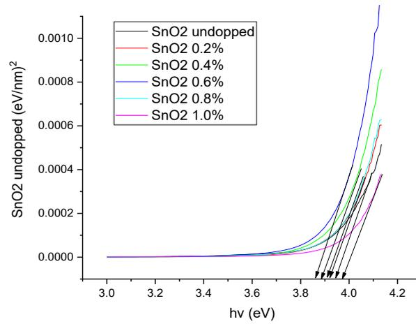
Fig. 2. Gap energy determination using Tauc's plot.
