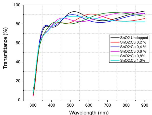
Fig. 1. Thin film transmittance for different doping percentage.
