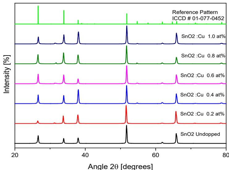
Fig. 2. XRD results for  $\text{SnO}_2$  doping with copper.
