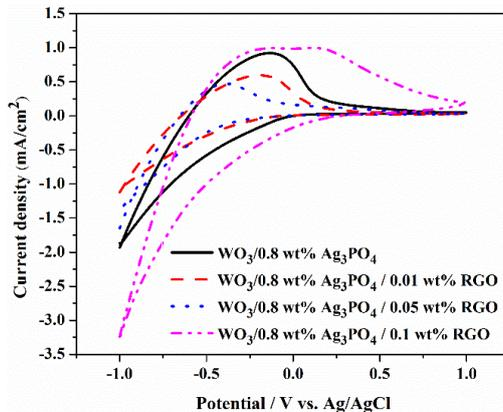
Fig. 4. Cyclic voltammograms of  $\text{WO}_3/0.8 \text{ wt}\% \text{ Ag}_3\text{PO}_4$ ,  $\text{WO}_3/0.8 \text{ wt}\% \text{ Ag}_3\text{PO}_4/0.01 \text{ wt}\% \text{ rGO}$ ,  $\text{WO}_3/0.8 \text{ wt}\% \text{ Ag}_3\text{PO}_4/0.05 \text{ wt}\% \text{ rGO}$  and  $\text{WO}_3/0.8 \text{ wt}\% \text{ Ag}_3\text{PO}_4/0.10 \text{ wt}\% \text{ rGO}$  films in  $0.5 \text{ M H}_2\text{SO}_4$  solution at a scan rate of  $100 \text{ mVs}^{-1}$ .
