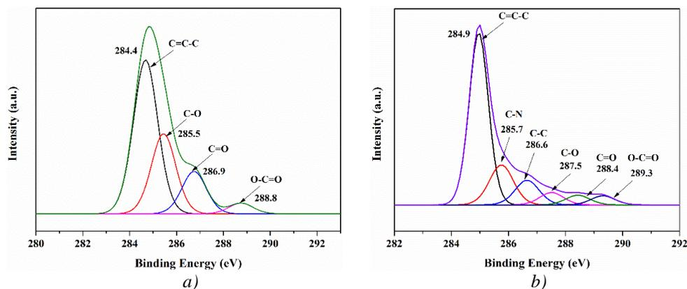
Fig. 3. The high-resolution XPS spectra of (a) C 1s on the  $\text{WO}_3/0.8 \text{ wt}\% \text{ Ag}_3\text{PO}_4/0.01 \text{ wt}\% \text{ rGO}$  film; (b) rGO sheet.
