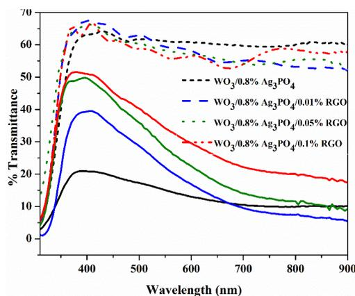
Fig. 5. UV-Vis transmittance spectra of  $WO_3/0.8 \text{ wt}\% Ag_3PO_4$ ,  $WO_3/0.8 \text{ wt}\% Ag_3PO_4/0.01 \text{ wt}\% rGO$ ,  $WO_3/0.8 \text{ wt}\% Ag_3PO_4/0.05 \text{ wt}\% rGO$  and  $WO_3/0.8 \text{ wt}\% Ag_3PO_4/0.10 \text{ wt}\% rGO$  films measured at 1.0 V (bleached state) and -1.0 V (colored state) in 0.5 M  $H_2SO_4$  solution.
