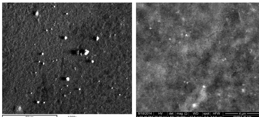
Fig. 4. Scanning Electron Microscopic images of silver nanoparticles biosynthesized by *Turbinaria turbinata*.
