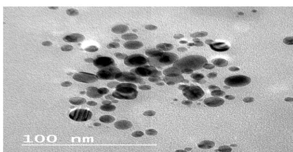
Fig. 3. Transmission Electron Microscopic image of silver nanoparticles biosynthesized by *Turbinaria turbinata*.
