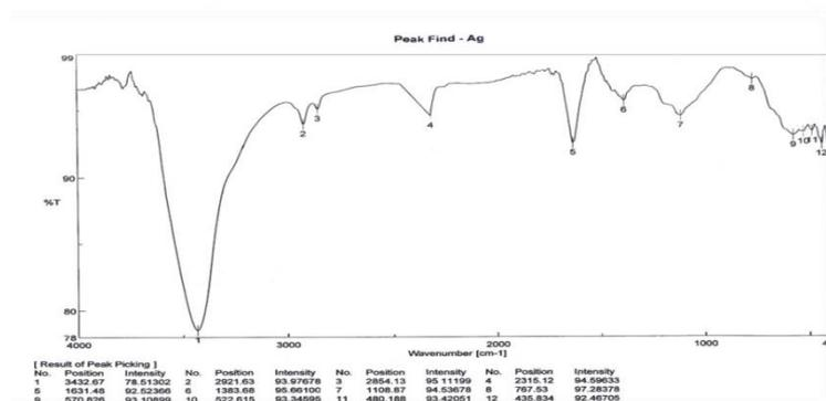
Fig. 7. Fourier transform infrared spectroscopic data of AgNPs biosynthesized by *Turbinaria turbinata*.
