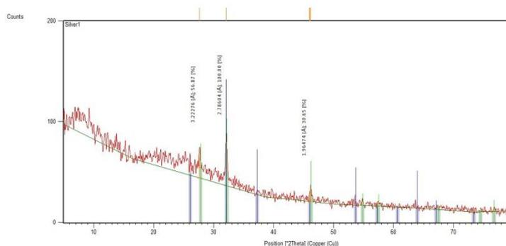
Fig. 5. X-ray diffraction analysis of silver nanoparticles biosynthesized by *Turbinaria turbinata*.
