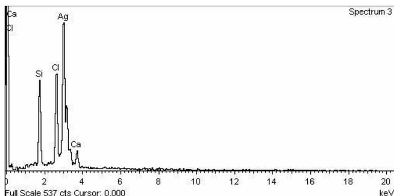
Fig. 6. Energy-dispersive X-ray analysis of AgNPs biosynthesized by *Turbinaria turbinata*.
