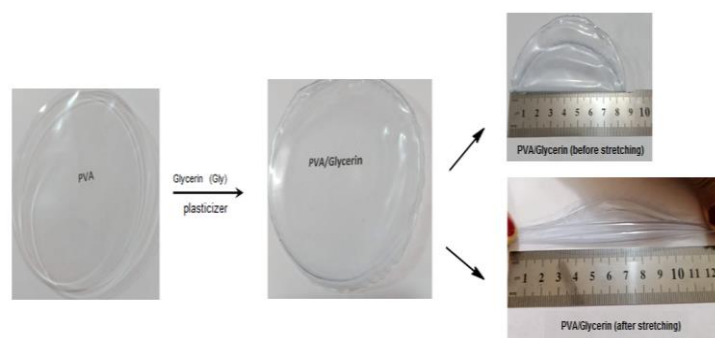
Fig.1. Digital photographs of a ductility experiment on PVA/3mL glycerin.
