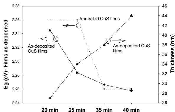
Fig. 3 Estimated band gaps of CuS films, and the thickness as a function of deposition time.
