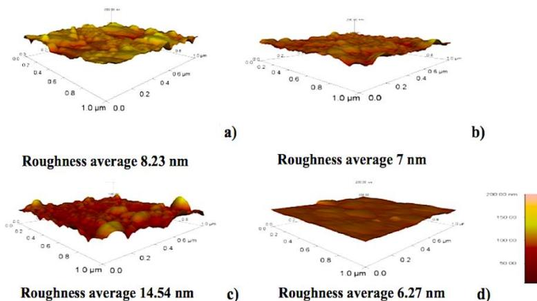
Fig. 4 AFM images of the samples: a) As-deposited b) with annealing process, both obtained at 25 min; c) As-deposited and d) with annealing process both obtained at 35 min.
