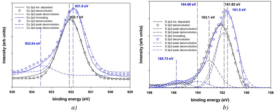
Fig. 5 XPS spectra of a) Cu 2p<sub>3/2</sub> and b) 2p<sub>1/2</sub> in the CuS films deposited at 35 min.
