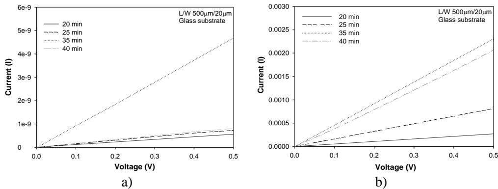
Fig. 6 Current-Voltage characteristics of CuS films a) As-deposited and b) Annealing
