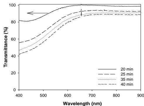
Fig. 2 Transmittance spectra of CuS films as deposited.
