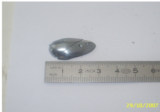
Fig. 1. Ingot of Sb_2S_3 after synthesized.
