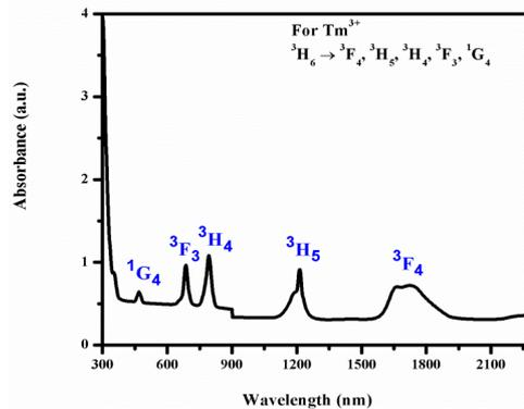
Fig. 4. UV–vis–NIR absorption spectrum of TNZ: Tm glass.
