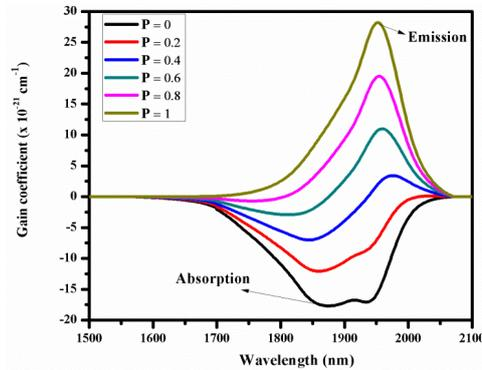
Fig. 6. The gain coefficient of the transition  ${}^3F_4 \rightarrow {}^3H_6$  for TNZ: Tm glass.
