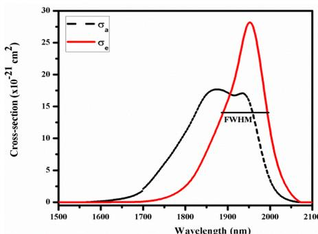
Fig. 5. absorption cross-sections  $\sigma_a(\lambda)$  and stimulated emission cross-sections  $\sigma_e(\lambda)$  of the transition  ${}^3H_6 \leftrightarrow {}^3F_4$  in TNZ: Tm.
