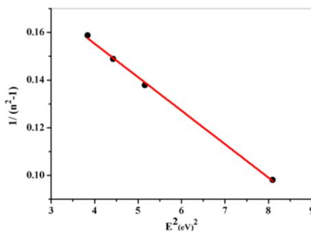
Fig.2: Dependency of the refractive index on the photon energy (illustrated as  $1/(n^2-1)$  vs.  $(E)^2$ ) of the TNZ glass doped with  $Tm^{3+}$  ions
