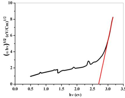
Fig. 3.  $(\alpha hv)^{1/2}$  as a function of  $hv$  for the TNZ doped with  $Tm^{3+}$  ions.
