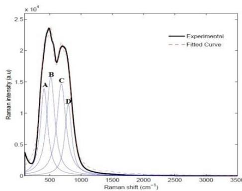
Fig. 7. Deconvoluted Raman spectra of TNZ: Tm glass.
