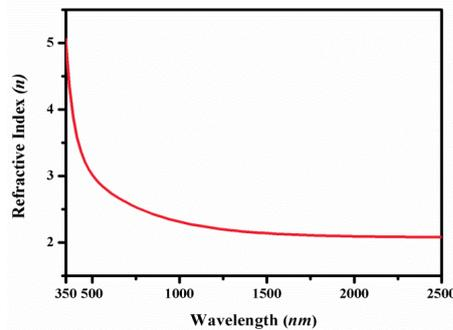
Fig. 1. Variation of refractive index as a function of wavelength for the TNZ doped with Tm<sup>3+</sup> ions.
