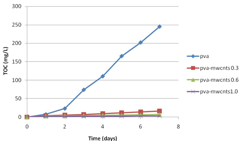
Graph 1: Effect of surface modified MWCNTs content loading on the TOC concentration.
