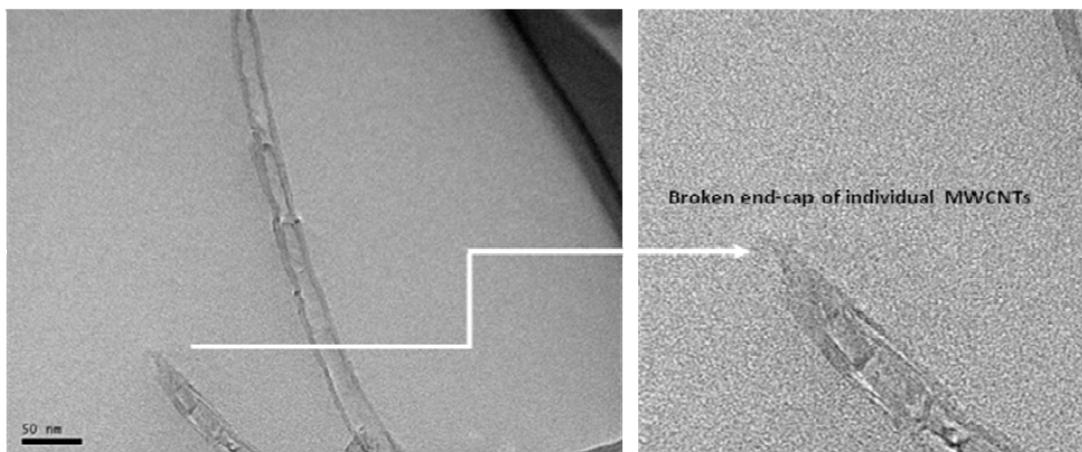
Fig. 2. Uncapping of MWCNTs end-tip
