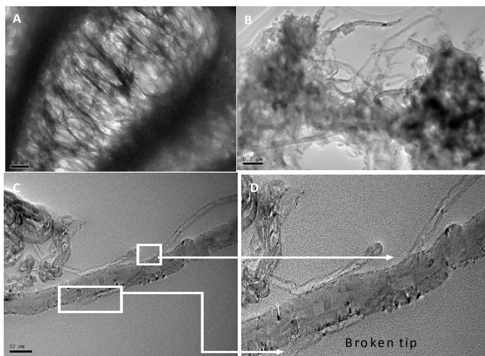
Fig. 1. (A) MWCNTs-PVA mixture (B) MWCNTs floss in PVA matrix (C) Pull out effect on MWCNTs-PVA mixture (D) Defect site of MWCNTs-PVA mixture.
