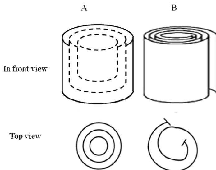
Fig. 3. Illustration of (a) Russian doll structure and (b) Swiss roll structure
