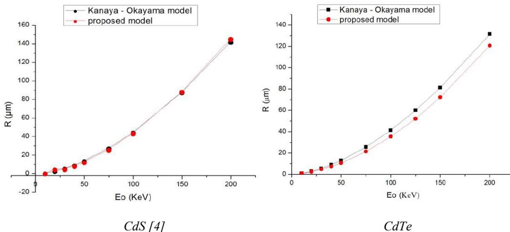
Fig. 1. Stopping range of electrons for CdS and CdTe materials as function of acceleration energy.
