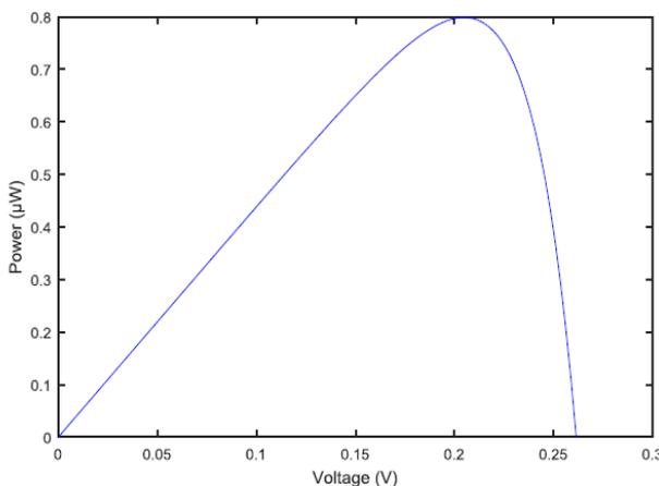
Fig. 6. Power voltage ( $P$ - $V$ ) for CdS/CdTe.
