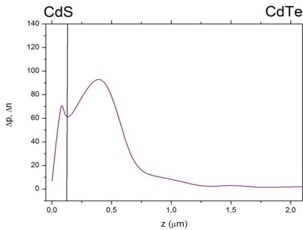
Fig. 3. The distribution of the concentration of electron-hole pairs generated by inelastic collisions of the incident electron with CdS/CdTe.
