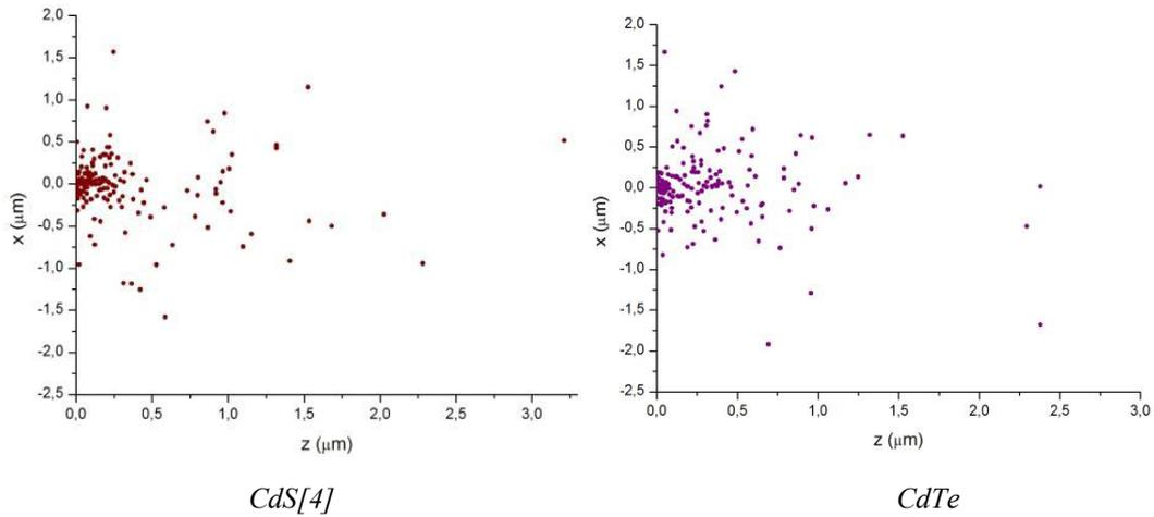
Fig. 2. The spatial distribution of electron-hole pairs generated as a function of depth in CdS [4] and CdTe For average energy 17 KeV.
