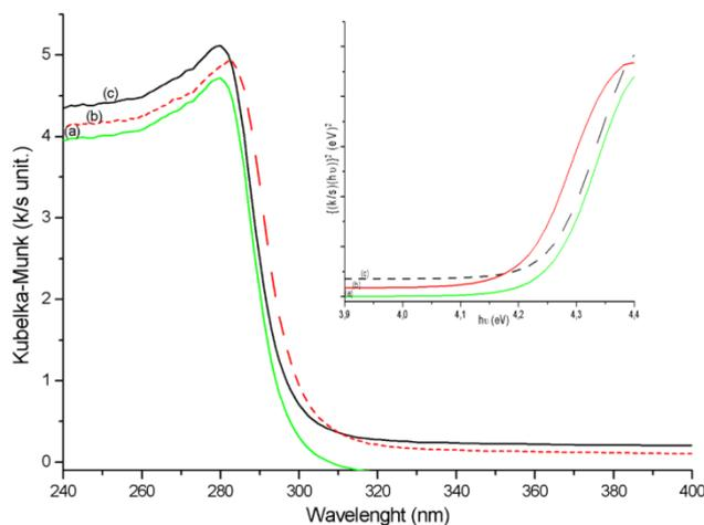
Fig. 6. Absorption spectra of heated  $ZnTa_2O_6$  at  $1100^\circ C$ : (a)  $pH=12.5$ ; (b)  $pH=10.5$  and (c)  $pH=7$ . Plot of  $\{(k/s)hv\}^2$  vs.  $hv$  (energy) of heated  $ZnTa_2O_6$  at  $1100^\circ C$ : (a)  $pH=12.5$ ; (b)  $pH=10.5$  and (c)  $pH=7$
