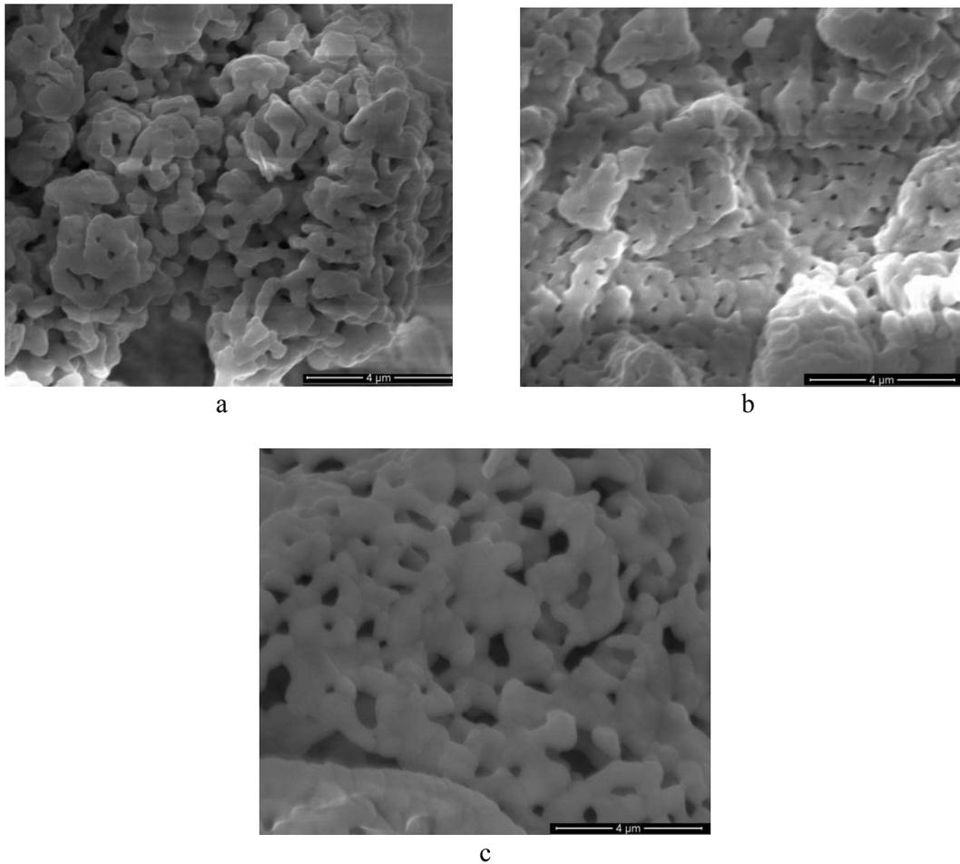
*Fig. 3 The SEM of  $ZnTa_2O_6$  powders obtained with different pH values heated at  $1100^\circ C$ .
