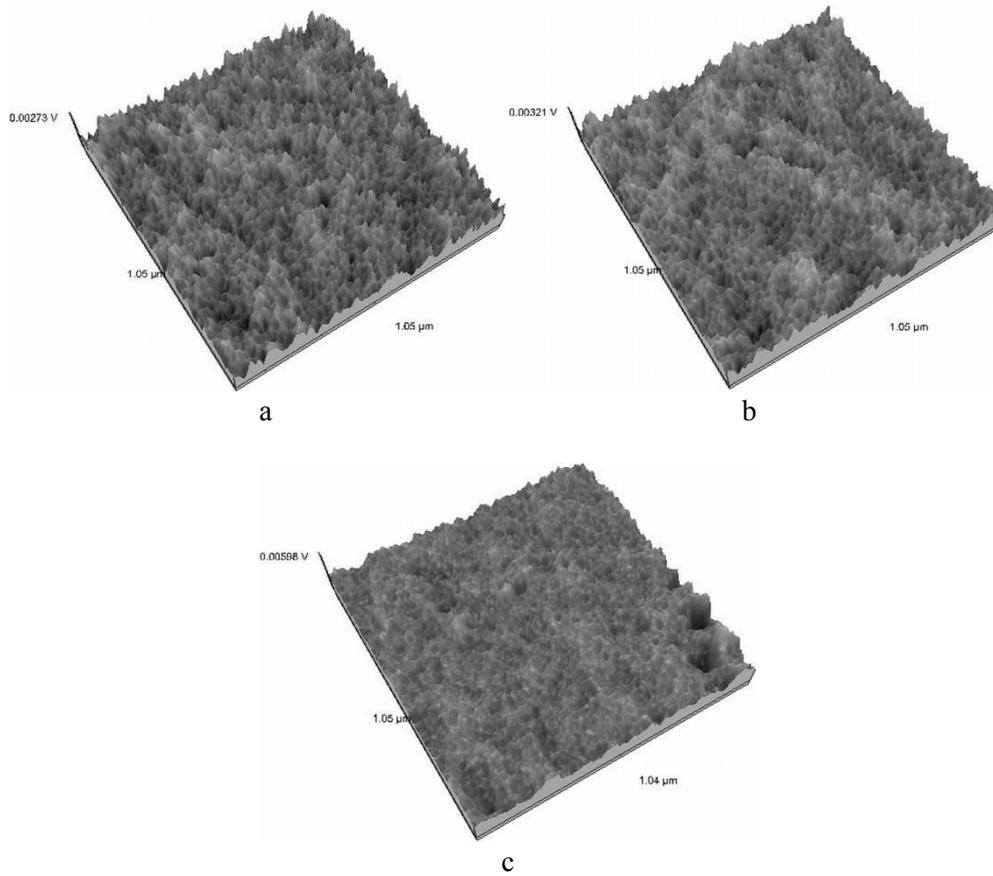
Fig. 4 AFM images of heated  $ZnTa_2O_6$  at  $1100\text{ }^\circ\text{C}$  powders, different pH values. (a) pH=12.5, (b) pH= 10.5, (c) pH= 7
