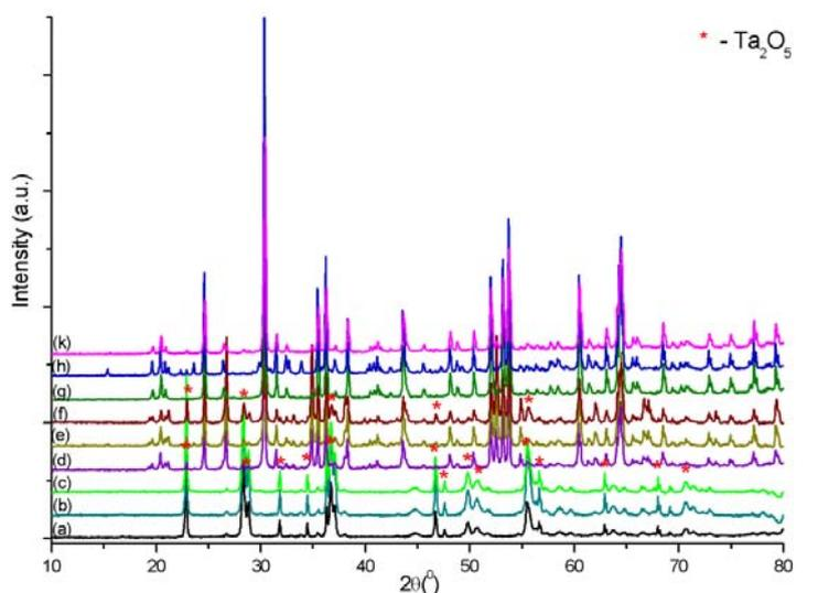
Fig.1 The XRD patterns of  $ZnTa_2O_6$ : (a) un- heated pH=12.5; (b) un- heated pH=10.5, (c) un- heated pH=7; (d) heated 1000 °C pH=12.5; (e) heated 1000 °C pH=10.5; (f) heated 1000 °C pH=7; (g) heated 1100 °C pH=12.5; (h) heated 1100 °C pH=10.5; (k) heated 1100 °C pH=7
