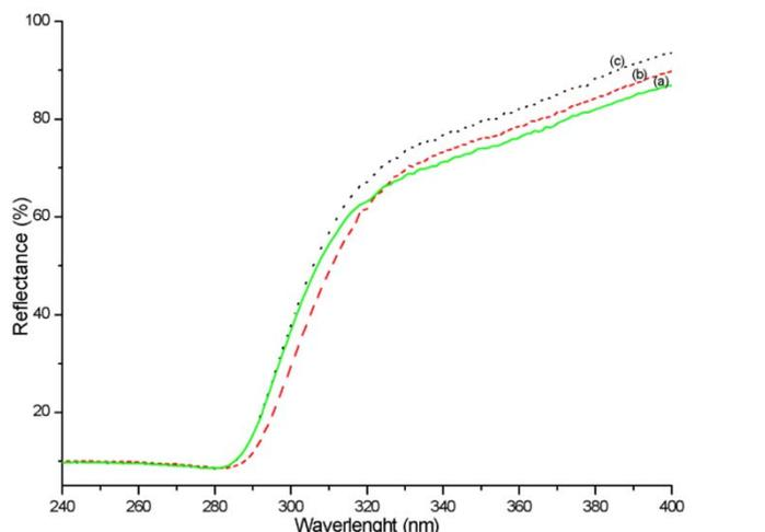
Fig. 5. Diffuse reflectance spectra of heated  $ZnTa_2O_6$  at  $1100^\circ C$ :
