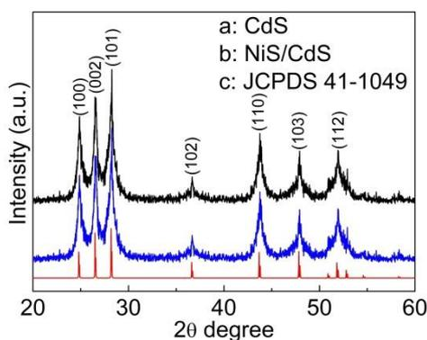
Fig.1 XRD patterns of CdS and NiS/CdS nanoparticles
