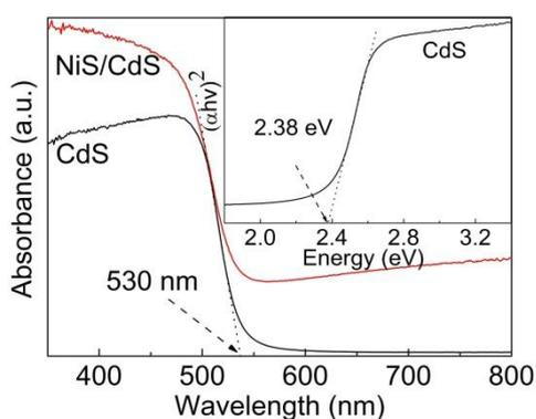
Fig.3 Diffuse reflectance spectra of CdS and NiS/CdS. Inset was the estimated band gap for CdS by Kubelka-Munk function
