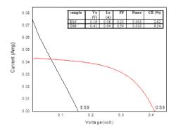
Fig. 6. I-V characteristics of fabricated photovoltaic cells using Alizarine red dye.
