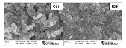
Fig.4.FE SEM image of SnO<sub>2</sub> nanostructure.
