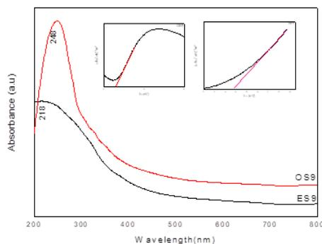
Fig. 3. UV- DRS and (inset) the corresponding  $(ahv)^2$  versus photon energy  $(h\nu)$  plot.
