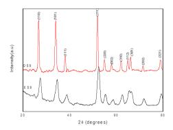
Fig. 2. XRD pattern of Synthesized SnO<sub>2</sub> nanostructure.
