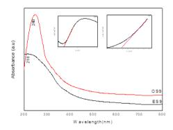
Fig. 3. UV- DRS and (inset) the corresponding  $(\alpha hv)^2$  versus photon energy (hv) plot.
