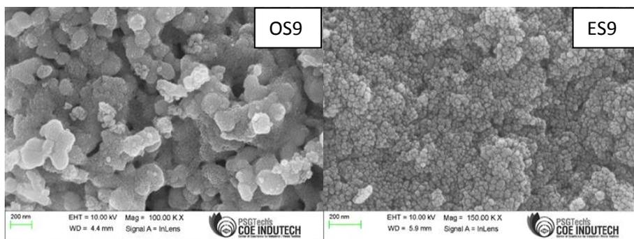
Fig.4.FE SEM image of  $\text{SnO}_2$  nanostructure.
