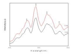
Fig.5.PL spectra of SnO<sub>2</sub> nanostructure.
