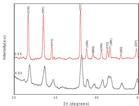
Fig. 2. XRD pattern of Synthesized  $\text{SnO}_2$  nanostructure.
