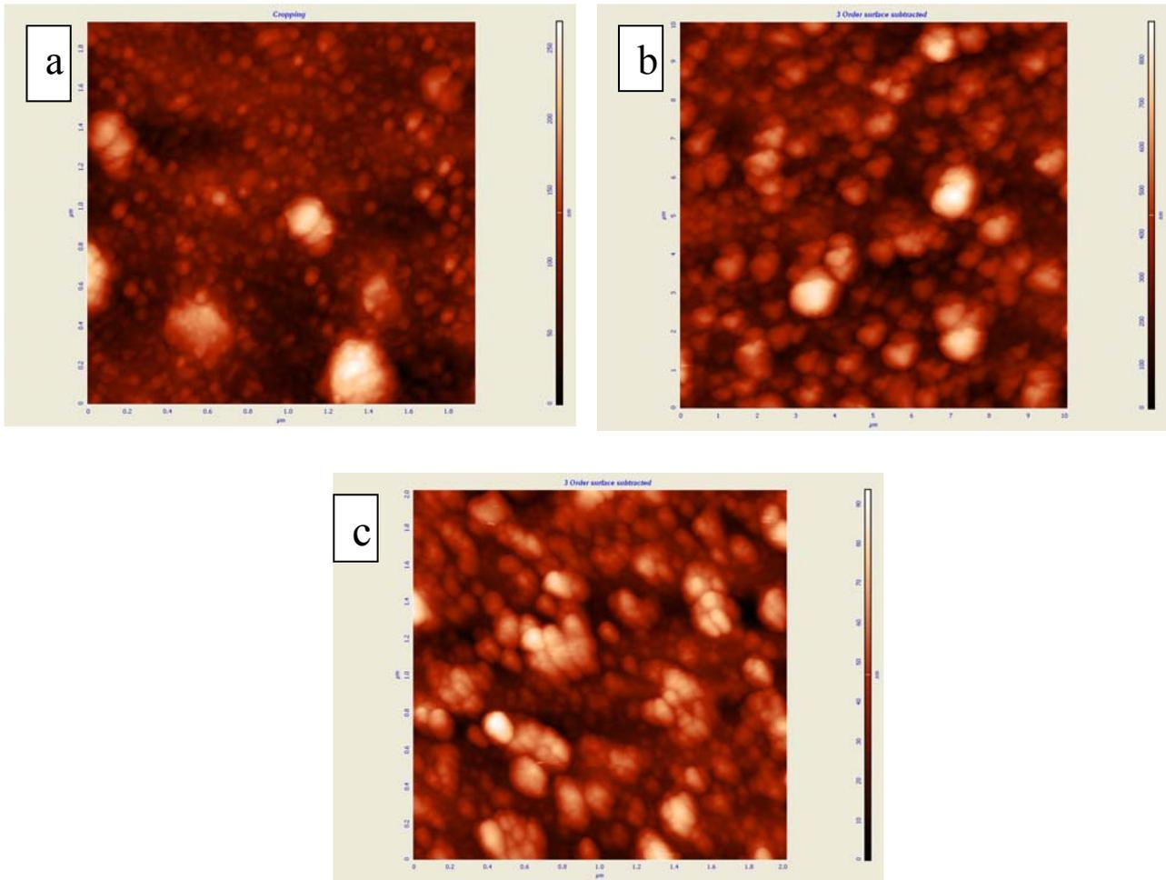
Fig. 2. Surface topography of lead sulphide thin films formed at different flux density (a)  $2.5 \text{ J/cm}^2$  (b)  $3.5 \text{ J/cm}^2$  and (c)  $4.16 \text{ J/cm}^2$
