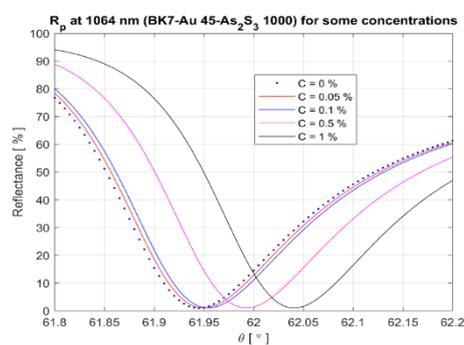
Fig. 4. Reflectance vs. incidence angle at different concentrations.
