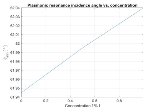
Fig. 5. Plasmonic resonance incidence angle vs. concentration.
