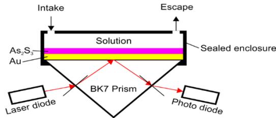
Fig. 1. *E. coli* detector schematic layout.
