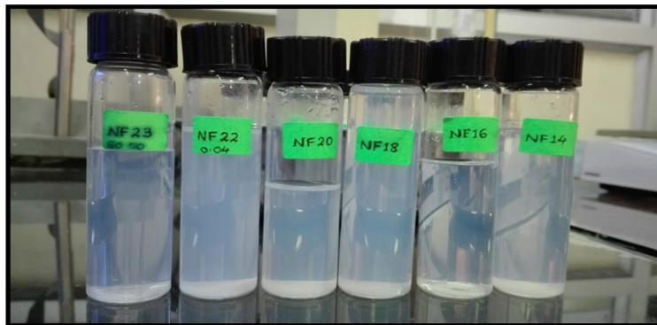
Fig. 3. Nanofluids with 0.02% TiO<sub>2</sub> and different ratio of dH<sub>2</sub>O and EG/PEG.
