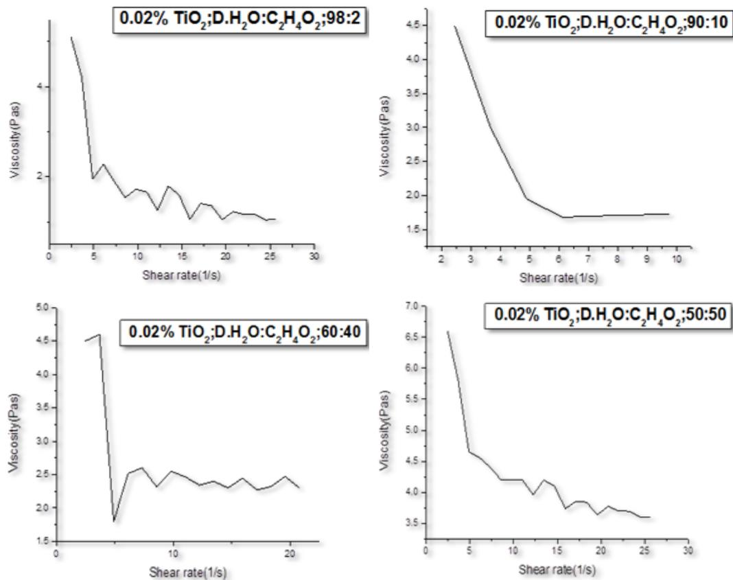
Fig. 5. (a-d) Rheology behavior for 0.02 wt % TiO<sub>2</sub> nanofluid with various ratio of dH<sub>2</sub>O:EG.
