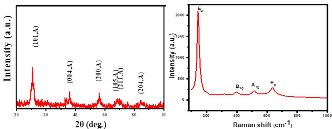
Fig. 1. (a) Powder XRD pattern of  $\text{TiO}_2$  Nanoparticles with major anatase phase (b) Raman spectrum of hydrothermal method prepared nanoparticle of  $\text{TiO}_2$ .
