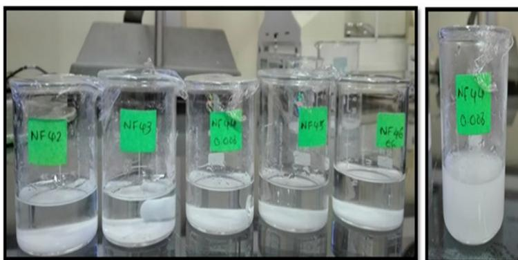
Fig. 4. (a) The comparative nanofluid formation with the addition of PEG and last image shows unclear nanofluid formation without the addition of PEG in commercial  $\text{TiO}_2$  nanoparticle.
