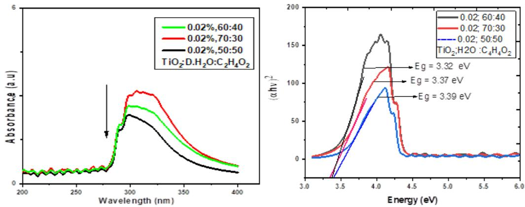
Fig. 2. (a) UV-Vis absorption spectra of titania nanoparticle at various dispersing medium (b) Band gap values of titania nanoparticle at various solvent condition.
