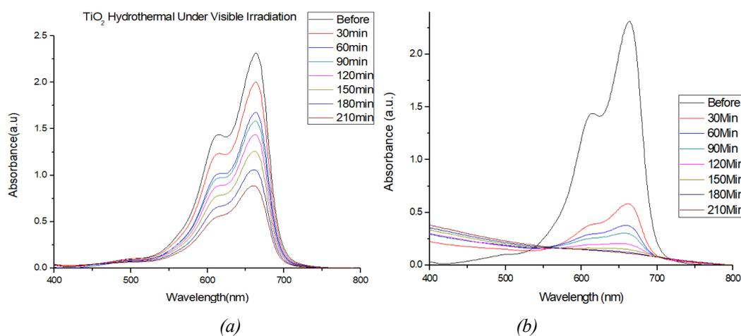
Fig. 7. Catalytic property of TiO<sub>2</sub> nanoparticle recovered from (a) water solvent (b) EG solvent.
