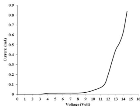
Fig. 4. I-V forward characteristics of ITO/PVV: PSS/ZnTe/Alq<sub>3</sub>with TiO<sub>2</sub>/Ni OLEDs.
