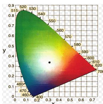
Fig. 7. The chromaticity-coordinates schemes of the PVV: PSS/ZnTe/Alq<sub>3</sub> with TiO<sub>2</sub> light-emitting device.
