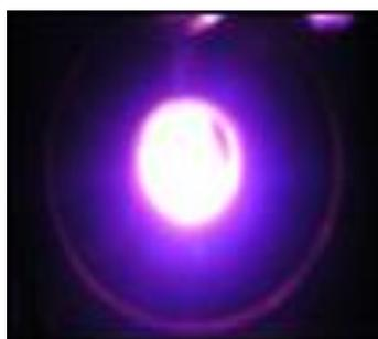
Fig. 6. A white light development imaging of PVV: PSS/ZnTe/Alq<sub>3</sub> with TiO<sub>2</sub> light-emitting device.
