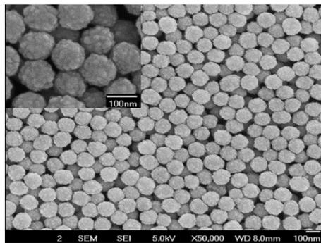
Fig. 3. Scanning electron microscope (SEM) of ZnTe NCs.
