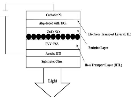
Fig. 1. Organic light-emitting device (OLED) ZnTe NCs based in a cross-sectional configuration.
