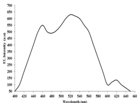
Fig. 5. Electroluminescence (EL) spectrum of PVV: PSS/ZnTe/Alq<sub>3</sub> with TiO<sub>2</sub> device.
