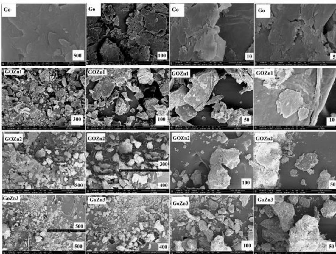
Fig. 2. FESEM micrographs of Graphene oxide /ZnO nanocomposites(a) GO (b) GOZn01 (c) GOZn02 (d) GOZn03.
