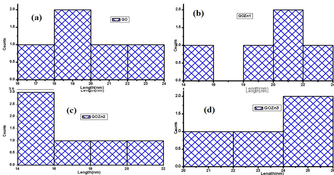
Fig. 3. Histograms of FESEM micrographs for calculating the average length of particles of (a) GO (b) GOZn1 (c) GOZn2 and (d) GOZn3.
