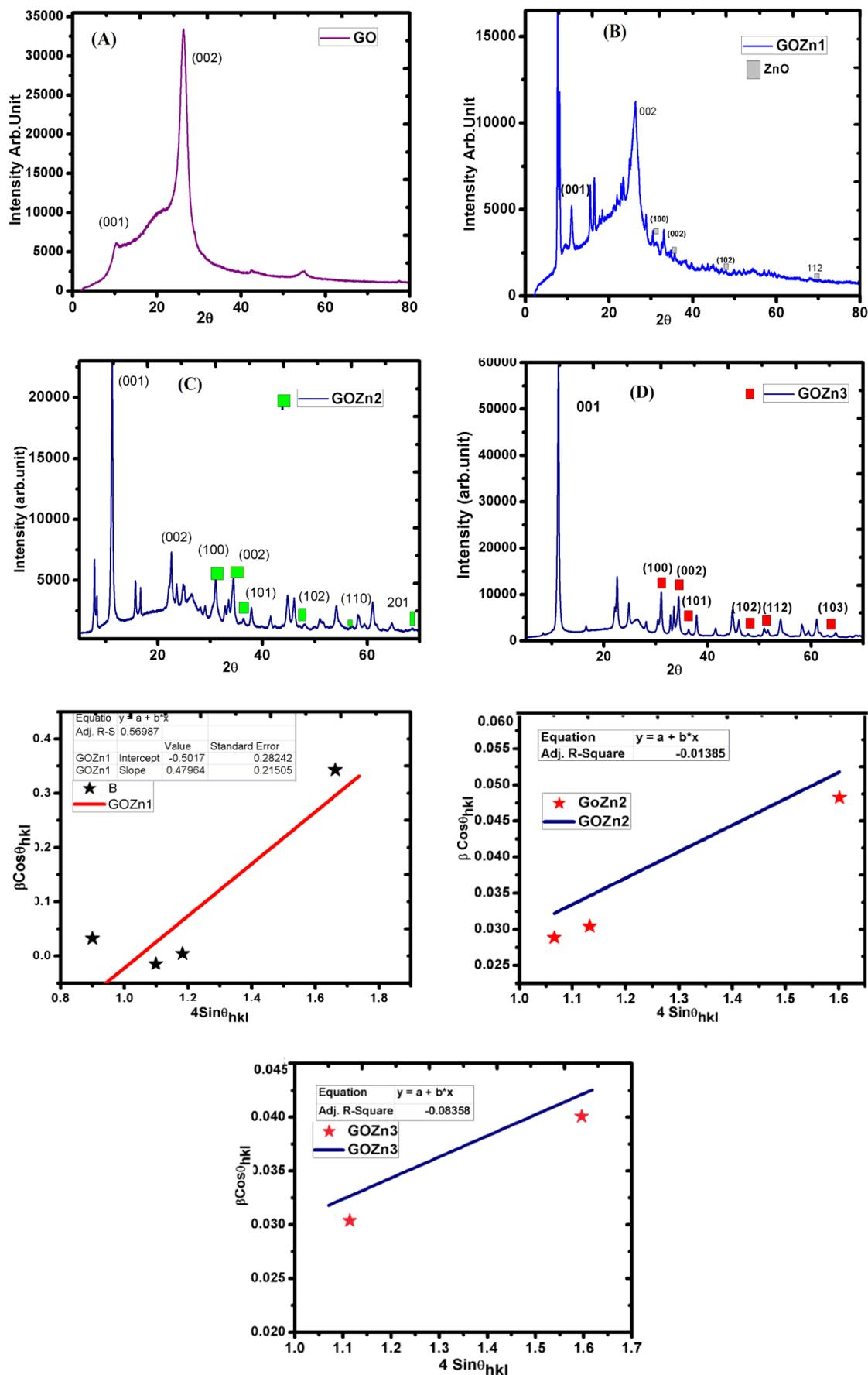
Fig. 1. XRD diffraction peaks and W-H plot of Graphene oxide Nanocomposites. (A) GO (B) GOZn1 (C) GOZn2 (D) GOZn3.
