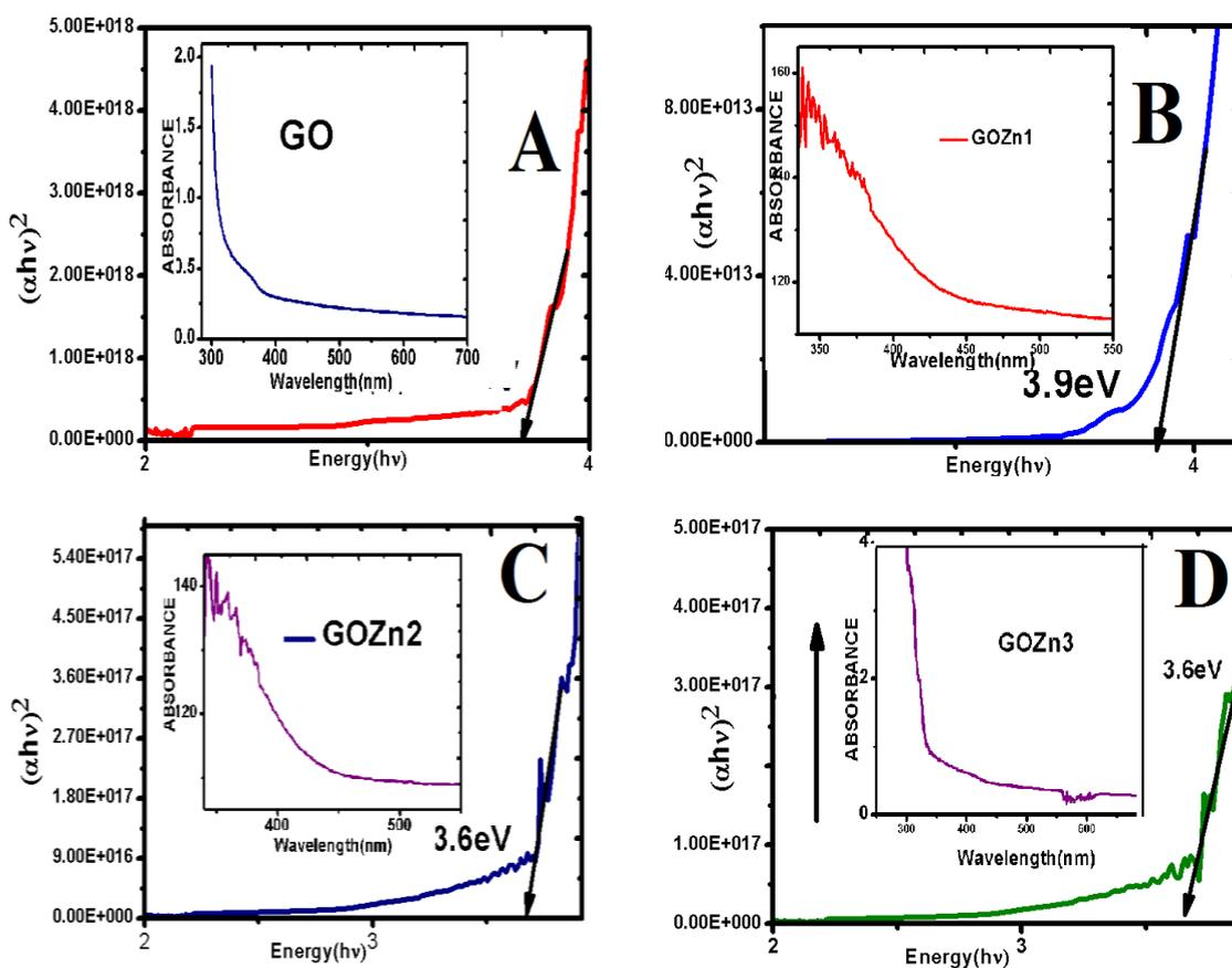
Fig. 5. UV-spectra and Tauc Plot of Graphene oxide and Graphene oxide/ZnO nanocomposites (a) GO (b) GOZn01 (c) GOZn02 (d) GOZn03.
