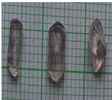
Fig. 2. As grown 0.1 M \text{AgNO}_3 doped \gamma -glycine crystal.
