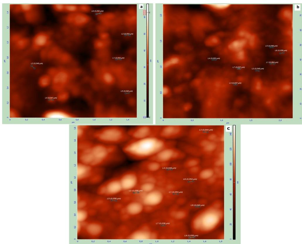
Fig. 2. Electron microscopic image of PP+Ag<sub>2</sub>S nanocomposites at various doses of  $\gamma$  irradiation of polypropylene powders a) 15kGy, b) 30 kGy, c) 50 kGy
