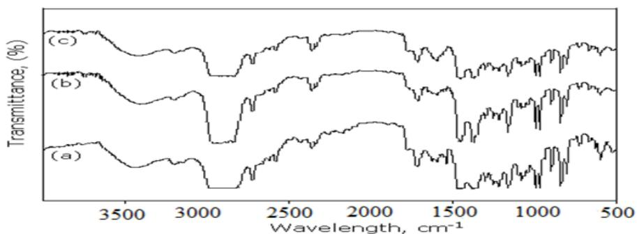
Fig. 5. IR spectra of nanocomposite PP/Ag<sub>2</sub>S prepared from previously  $\gamma$  rays irradiated polypropylene powders at 15 kGy, 30 kGy, 50 kGy
