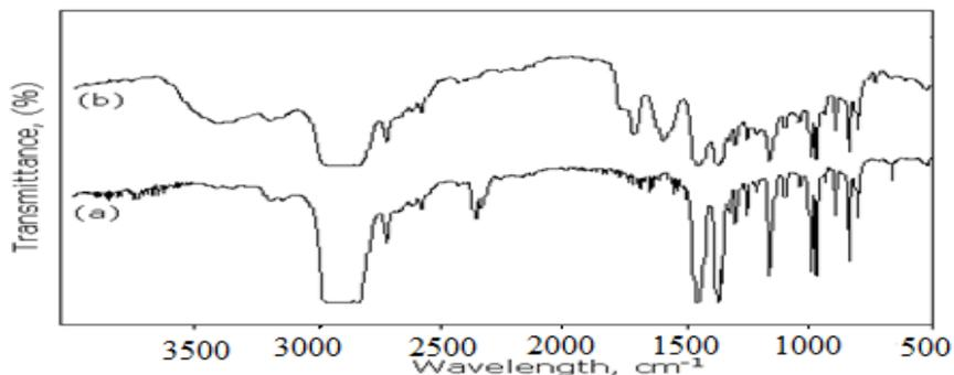
Fig. 4. IR spectrum of polypropylene (a) and pre-irradiated at 15 kGy (b)
