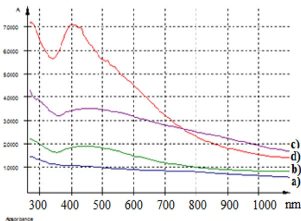
Fig.6 UV spectra of pure polypropylene film (a) and nanocomposites PP + Ag<sub>2</sub>S based on previously  $\gamma$  rays irradiated polypropylene powders at 15 kGy (d), 30 kGy (c), 50 kGy (b)
