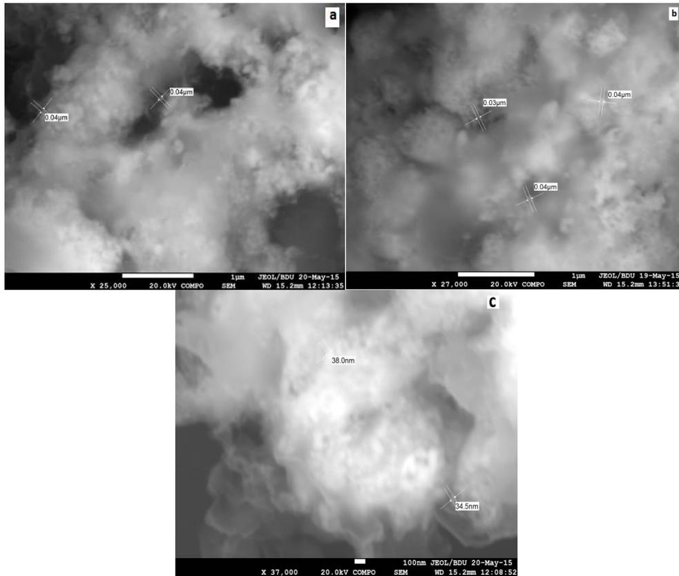
*Fig.1. Electron microscope image of nanocomposites based on PP + Ag<sub>2</sub>S at various doses  $\gamma$  irradiation of polypropylene powders a) 15kGy, b) 30 kGy, c) 50 kGy*
