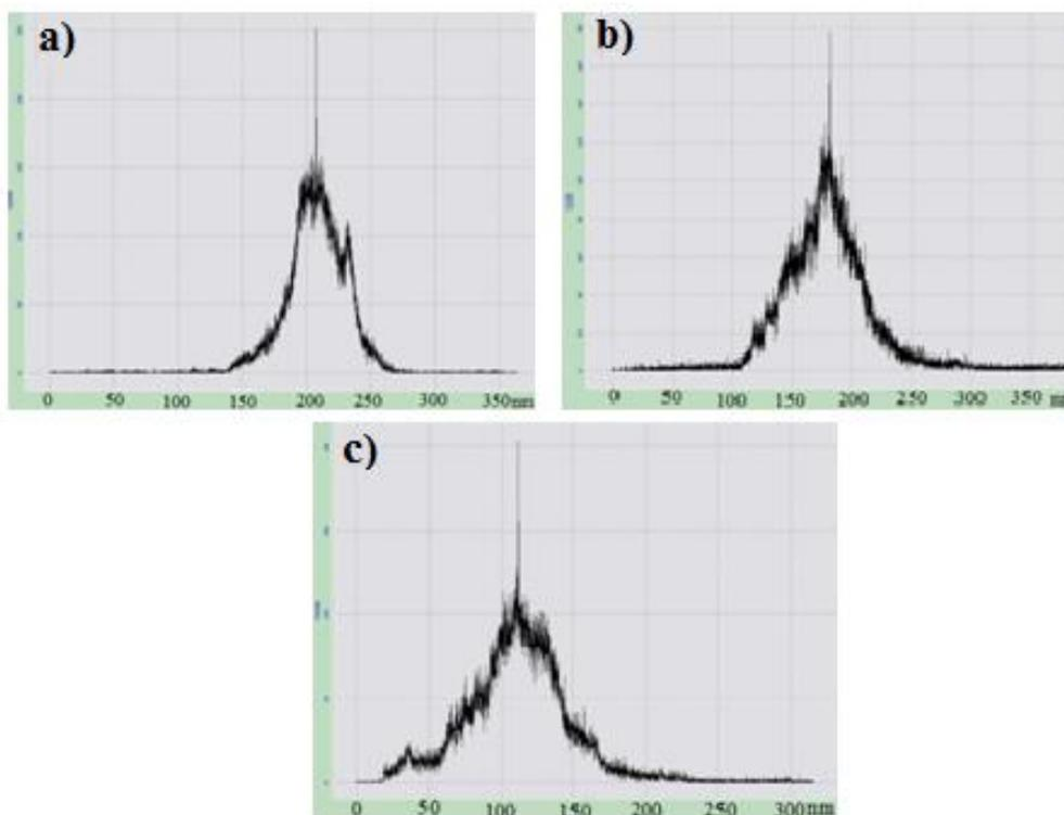
*Fig. 3. Histogram of the values of elements of the nanocomposite images PP + Ag<sub>2</sub>S obtained at different  $\gamma$  irradiation doses of polypropylene powders: a) 15kGy, b) 30 kGy, c) 50 kGy*
