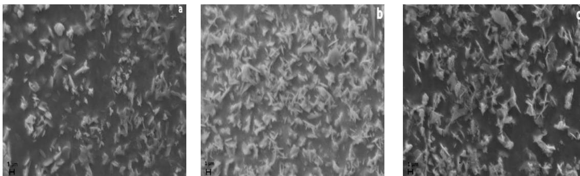
Fig. 3: SEM images of of annealed CTS films obtained with Cu/Sn ratios of (a) 1.82, (b) 2.03 and (C) 2.27
