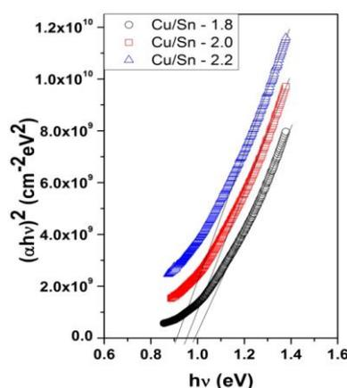
Fig. 4:  $(\alpha hv)^2$  versus  $hv$  plots of CTS films obtained with different Cu/Sn ratio by annealing the spray deposited films.
