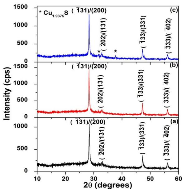
Fig. 1: XRD patterns of CTS films obtained with Cu/Sn ratios of (a) 1.82, (b) 2.03 and (c) 2.27.
