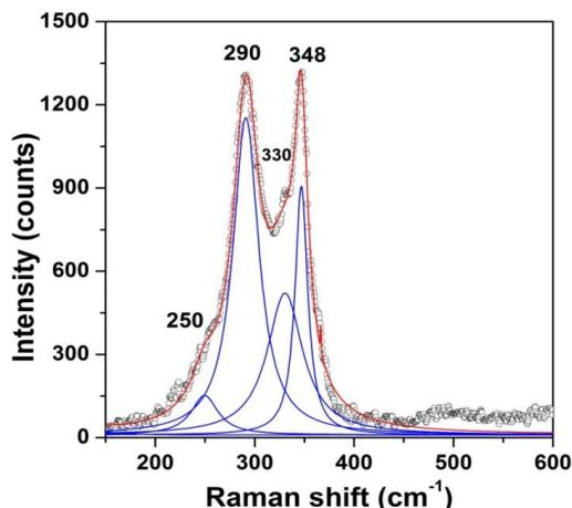
Fig. 2: Raman spectrum of Cu-correct CTS film obtained by annealing the spray deposited films
