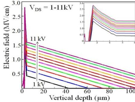
Fig. 2. Vertical depth dependent electric field distribution taken by cutting vertical half structure.
