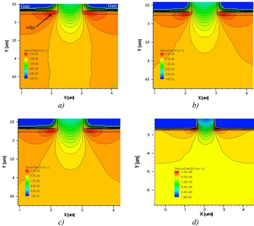
Fig. 3. 2D electric field distribution at different negative gate voltage (a) -18 V (b) -14 V (c) -10 V (d) -6 V.
