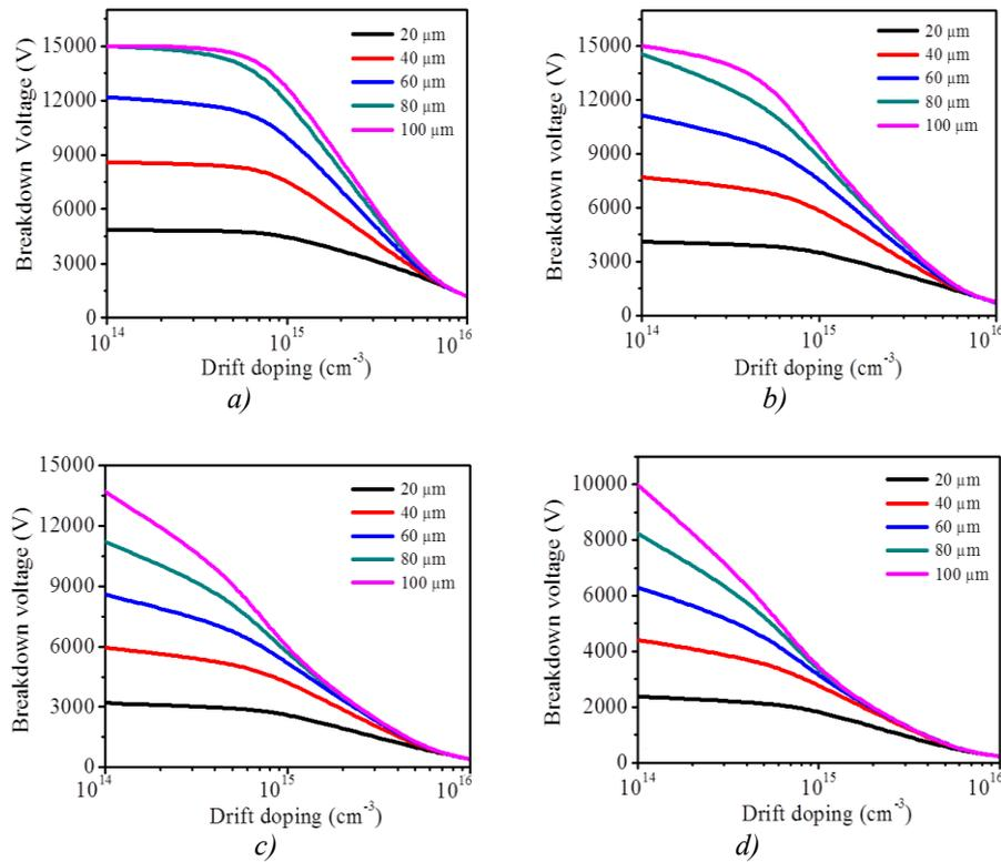
Fig. 5. Drift doping dependent breakdown voltage at various channels (a)  $W_{ch} = 0.6 \mu\text{m}$  (b)  $W_{ch} = 0.7 \mu\text{m}$  (c)  $W_{ch} = 0.8 \mu\text{m}$  (d)  $W_{ch} = 0.9 \mu\text{m}$  width under the negative gate bias of  $-30 \text{ V}$  with different drift layer thickness from  $20$  to  $100 \mu\text{m}$ .
