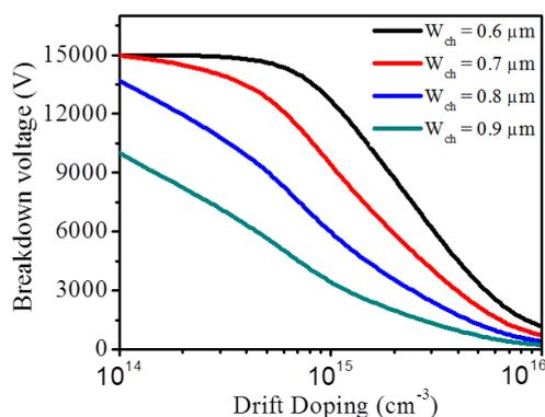
Fig. 6. Effect of drift doping with different channel with at drift layer thickness of  $100 \mu\text{m}$  gate bias of  $-30 \text{ V}$ .
