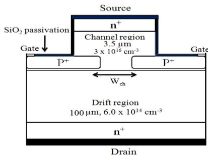
Fig. 1. Cross-sectional view of device structure.
