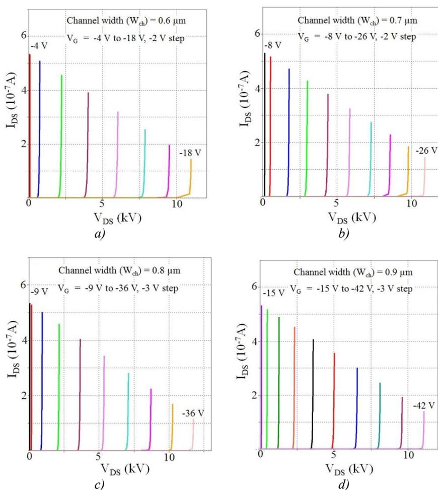
Fig. 4. Channel width dependent breakdown voltage characteristics of normally-on SiC VJFET at various negative voltages  $V_G$  (a)  $-4$  to  $-18\ \text{V}$  (b)  $-8$  to  $-26\ \text{V}$  (c)  $-9$  to  $-36\ \text{V}$  (d)  $-15$  to  $-42\ \text{V}$ .
