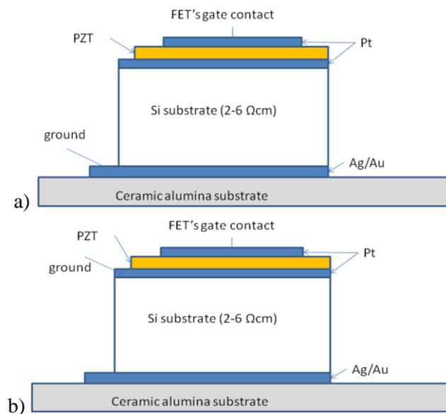
Fig. 2 a) connection with the Si substrate included in the measurement circuit, considering the entire Pt/Si/Ag/Au stack as bottom electrode for the PZT film; b) connection without the Si substrate included in the measurement circuit (ground contact on the Pt layer deposited on Si, gate contact on the top Pt electrode).
