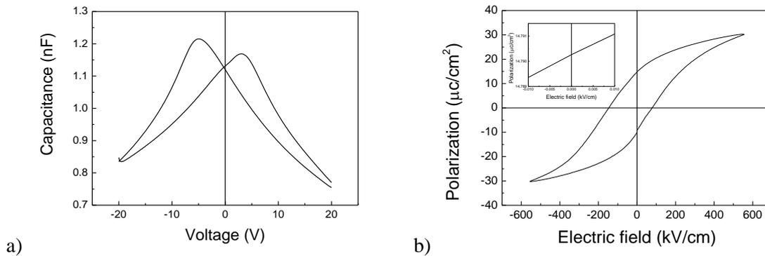
Fig. 5 a) the C-V characteristic of the PZT capacitor used as pyroelectric element on Pt/Si substrate; b) the hysteresis loop obtained for a PZT film deposited on Pt/Si substrate. The inset shows the polarization variation at low electric fields, around zero volts/cm.
