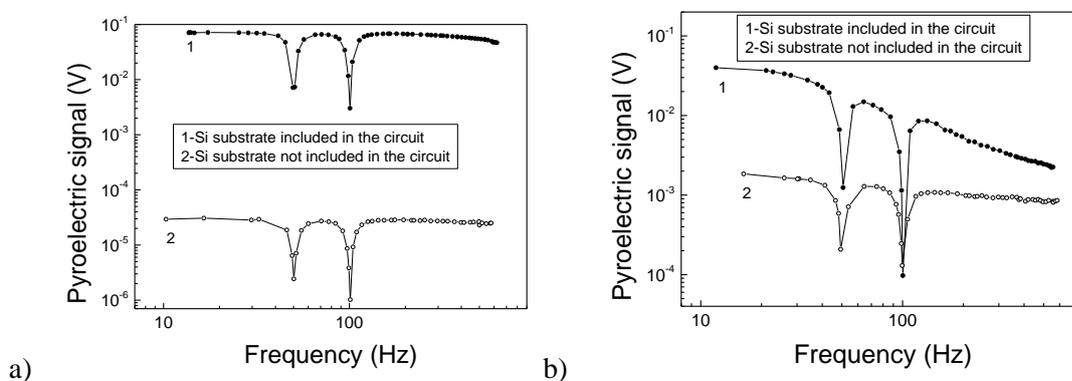
Fig. 6 Frequency dependence of the pyroelectric signal, with and without the Si substrate included in the measuring circuit, for a PZT-BiFeO<sub>3</sub> multilayer (a) and for AlN thin film (b). The PZT-BiFeO<sub>3</sub> multilayer was deposited by sol-gel. The AlN film was deposited by radio-frequency (RF) sputtering. The Si substrate was of the same quality as for the PZT films shown in Fig. 1.
