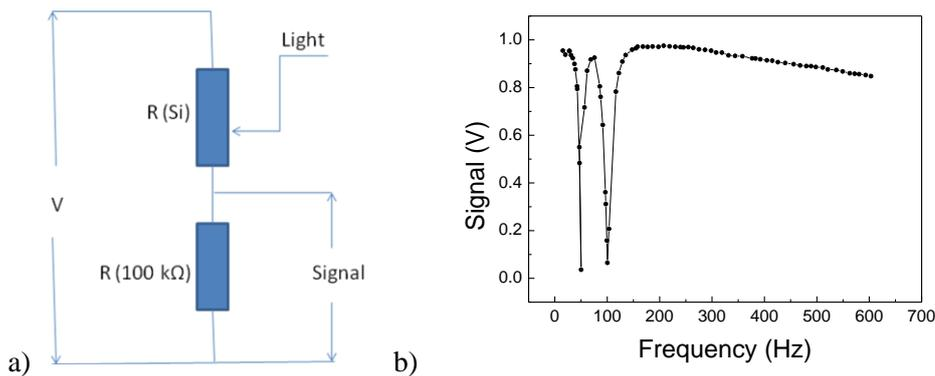
Fig. 4 a) set-up for photoconductivity measurement on Pt/Si substrate; b) the frequency dependence of the photoconductive signal obtained from the Pt/Si substrate.
