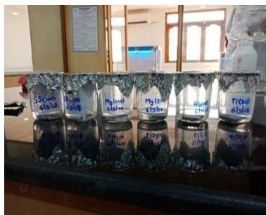
Fig. 1. Samples immersed in Simulated body fluid solution for Apatite formation test.
