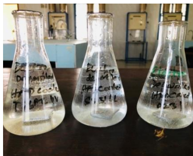
Fig. 3. Immersion testing of S316L, Ti6AL4V and AZ31 substrates.
