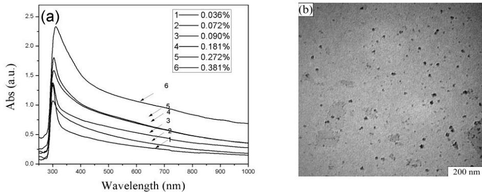
Fig.3: (a) UV-Vis spectra of Al nanofluids in different mass fraction concentrations. (b) TEM image of 0.090 % (w/w) Al NP suspended in ethylene glycol.
