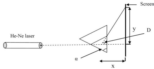
Fig.2: The experimental set up for measuring refractive index of liquids.
