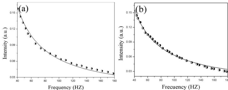
Fig.4: Intensity dependent on the frequency variations obtained by photoacoustic spectroscopy for (a) 0.036 % and (b) 0.090 % (w/w) Al NPs suspended in EG.
