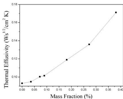
Fig.5: Variation of thermal effusivity versus mass concentration of Al NPs.
