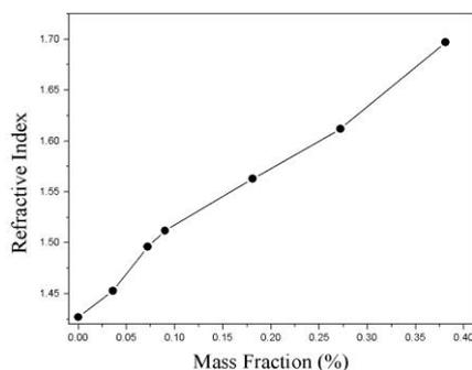
Fig.6: Variation of refractive index versus mass concentration of Al NPs.
