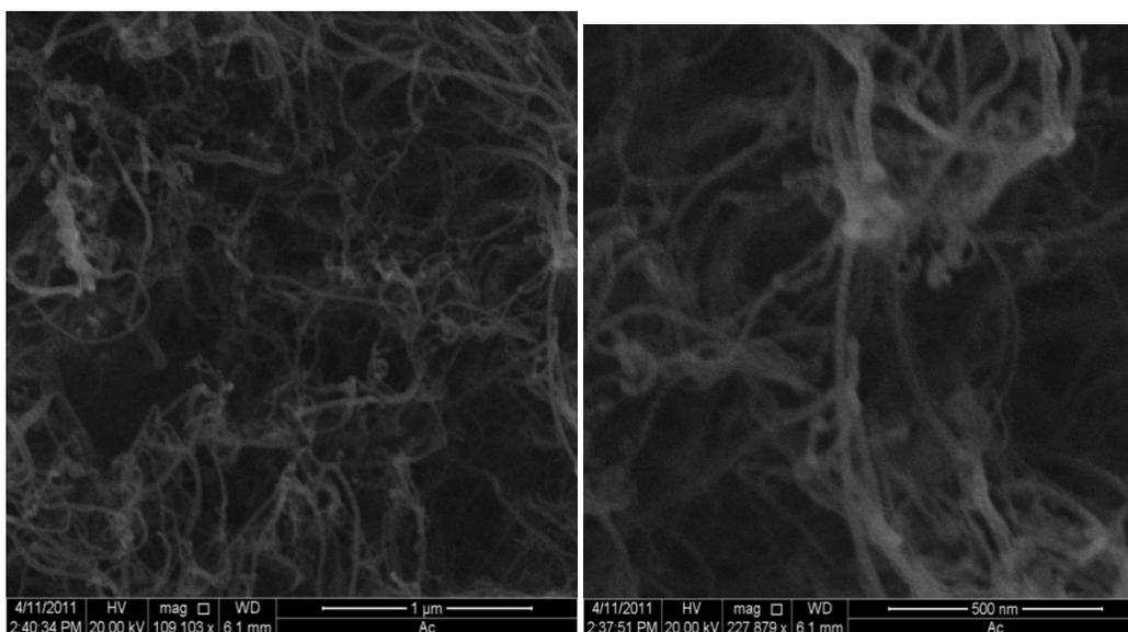
Fig. 1(a and b): FESEM images of MWCNTs deposited with platinum nanoparticles.
