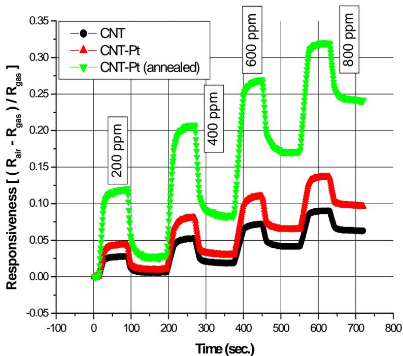
Fig. 5. Typical responsiveness of MWCNTs film sensor, MWCNTs deposited with platinum nanoparticles film sensor and MWCNTs deposited with platinum nanoparticles film sensor annealed at 400°C for 1 hours for different concentration of CO gas (200, 400, 600 and 800 ppm).
