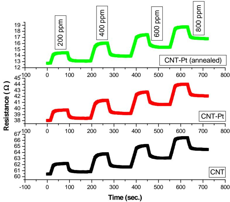
Fig. 3. Typical responses of MWCNTs film sensor, MWCNTs deposited with platinum nanoparticles film sensor and MWNTs deposited with platinum nanoparticles film sensor annealed at 400°C for 1 hour for different concentration of CO gas (200, 400, 600 and 800 ppm).
