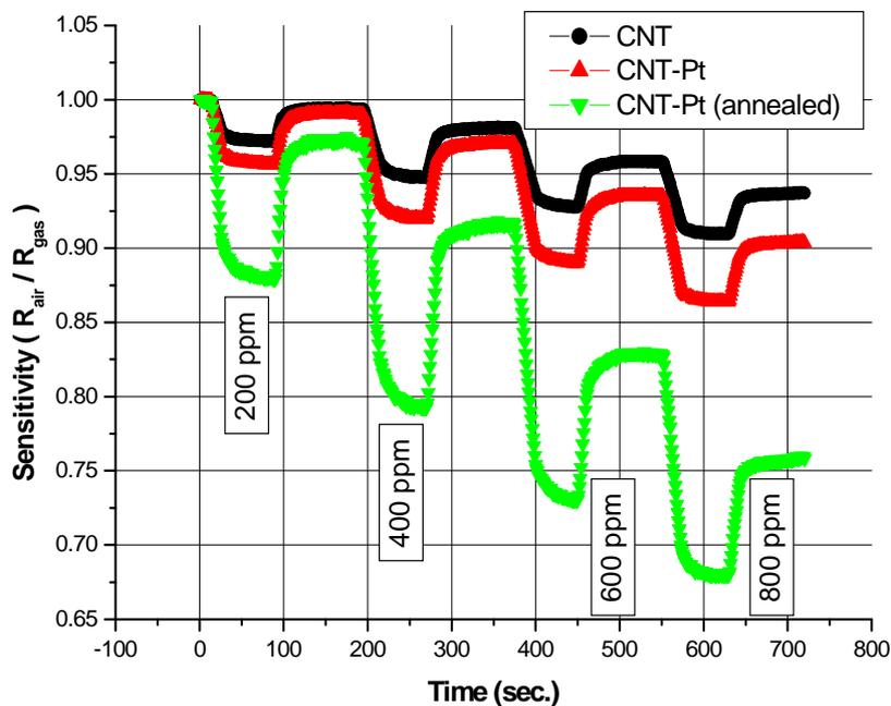
Fig. 4. Typical sensitivity of MWCNTs film sensor, MWCNTs deposited with platinum nanoparticles film sensor and MWCNTs deposited with platinum nanoparticles film sensor annealed at 400°C for 1 hours for different concentration of CO gas (200, 400, 600 and 800 ppm).
