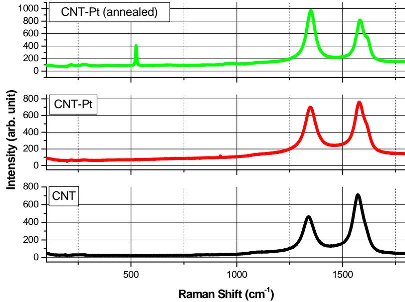
Fig. 2. Raman spectra of as-synthesized MWCNTs, MWCNTs deposited with platinum nanoparticles and MWCNTs deposited with platinum nanoparticles annealed at 400°C for 2 hours.
