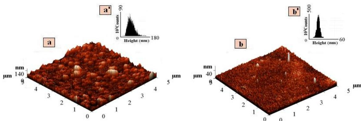
Fig. 3. Tapping mode of AFM images and histograms of immobilized collagen surfaces a) after C30; b) after PC30
