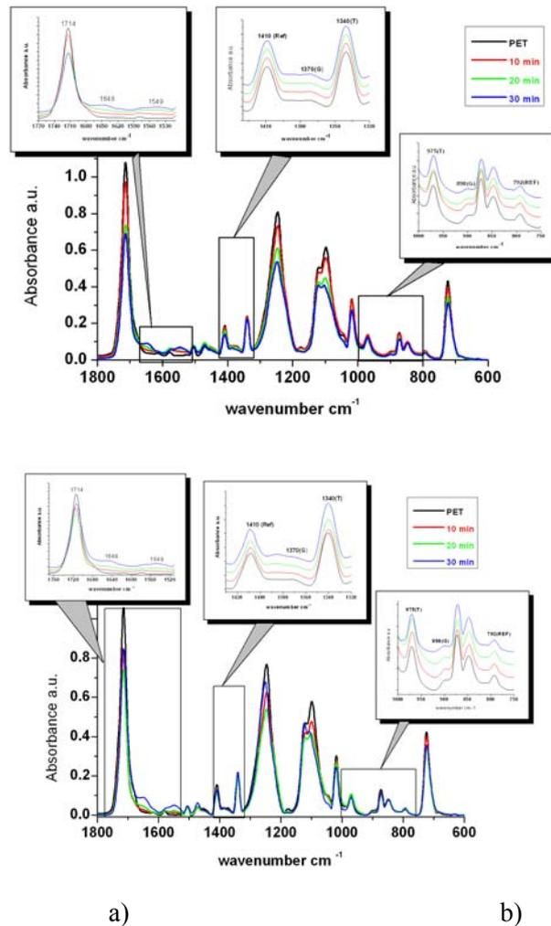
Fig. 1. FTIR measurements for a) chemical treatments; b) plasma and chemical treatments
