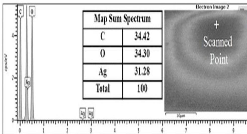
Fig. 1. EDX spectrum of Ag-ZnO nanocomposite.
