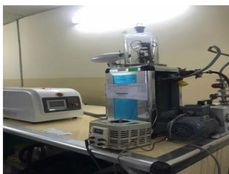
*Fig. 1 the system of the pulse laser deposition (pld)*
