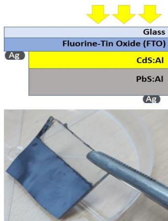
Fig. 1. Thin film solar cells CdS/PbS cross-sectional diagram and solar cell after the deposition of the PbS layer. The solar cell size is 5.0 x 3.0 cm.
