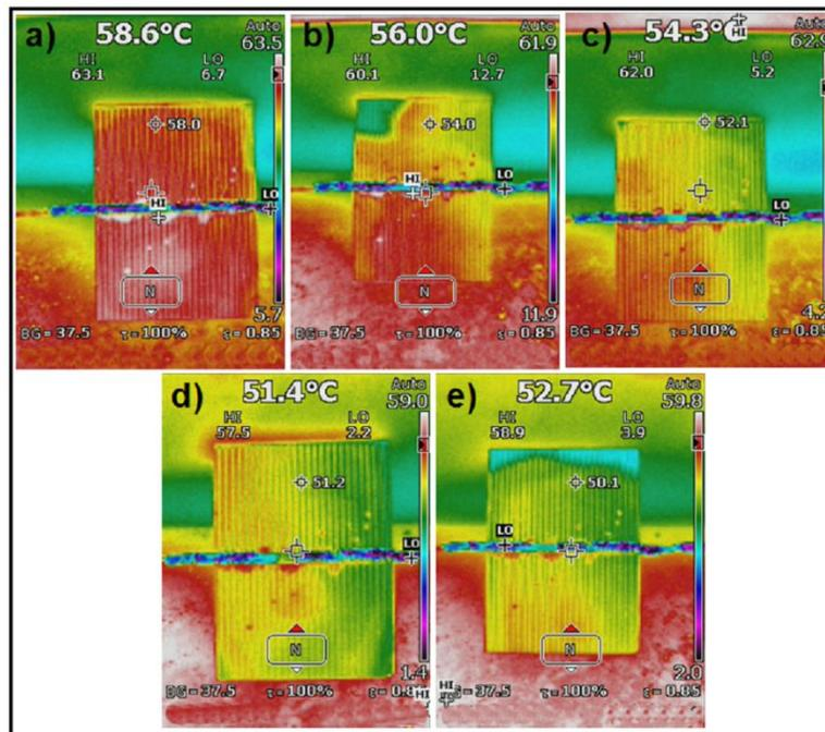
Fig. 11 (i) Temperature exploration of ZnS coated and bare polycrystalline Si solar cells under open source conditions.
