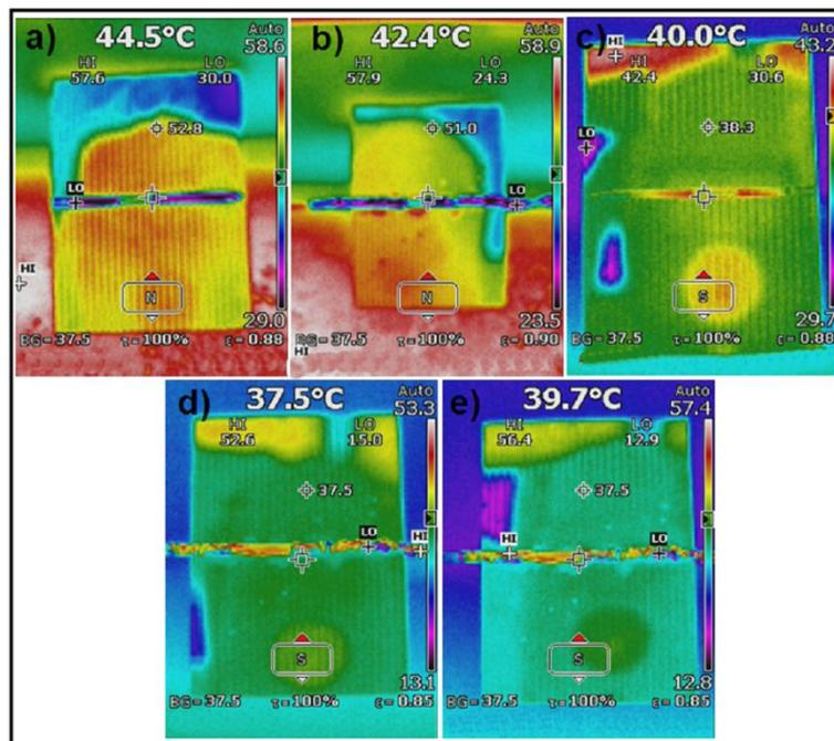
Fig. 11 (ii) Temperature exploration of ZnS coated and bare polycrystalline Si solar cells under closed source conditions.
