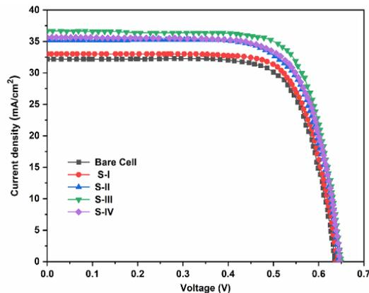
Fig. 8 I-V performance of bare cell and ZnS coated solar cell under open source conditions.
