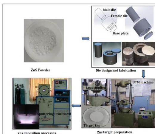
Fig. 1. ZnS target preparation and deposition processes.
