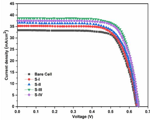
Fig. 10 I-V performance of bare cell and ZnS coated solar cell under controlled source conditions.
