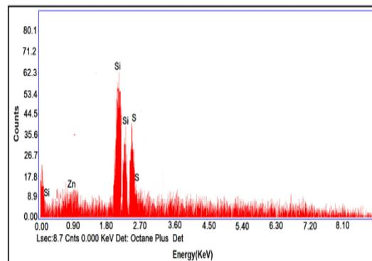
Fig. 5 EDAX of ZnS nano films deposited at S-III min duration on solar cell.
