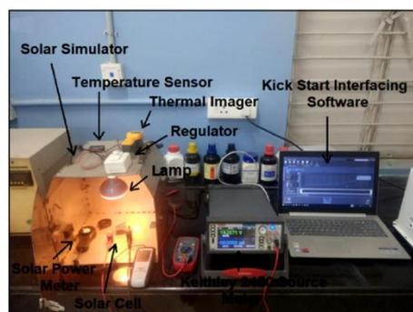
Fig. 9 Controlled source condition experimental setup.
