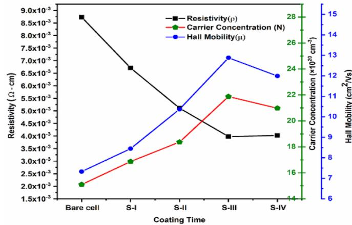
Fig. 7. Electrical resistivity ( $\rho$ ), carrier concentrations ( $N$ ) and Hall mobility ( $\mu$ ) of the uncoated cell and ZnS coated solar cells with different sputtering periods of S-I to S-IV min.
