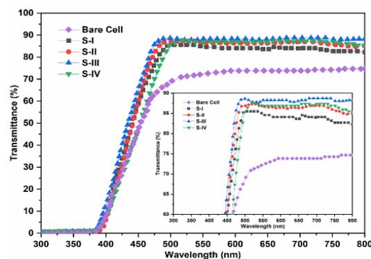
Fig. 6 Optical transmittance characteristics of ZnS coated and bare polycrystalline Si solar cells
