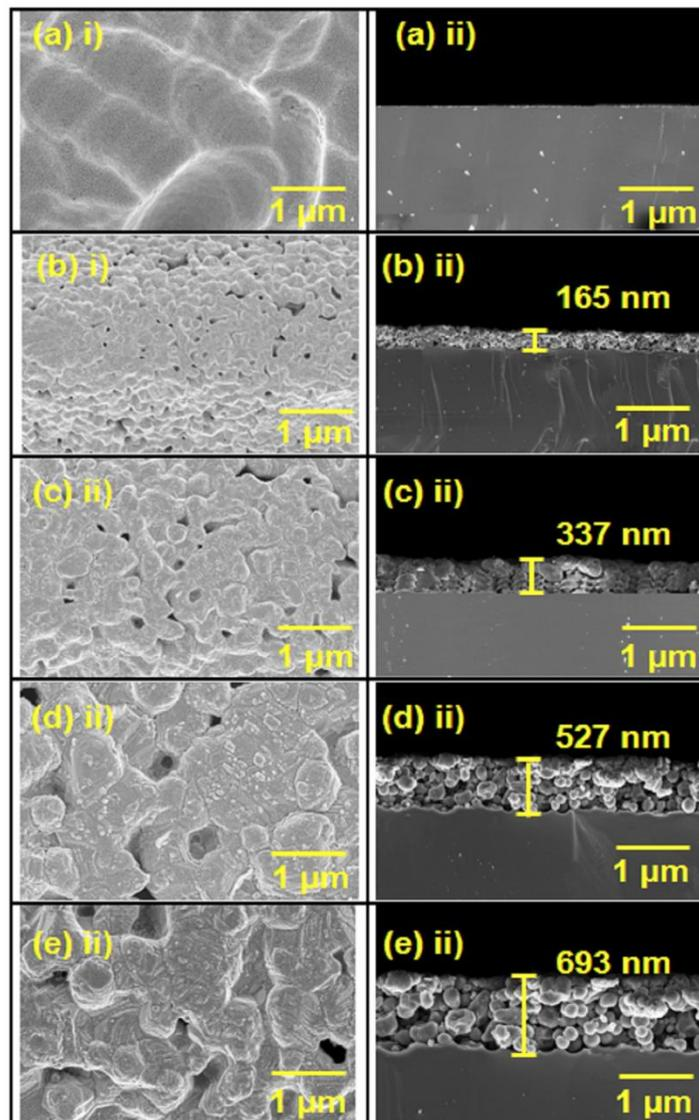
Fig. 4 FE-SEM image of bare cell a) (i & ii) and ZnS coated solar cells; b) S-I (i & ii), c) S-II (i & ii), d) S-III (i & ii), and e) S-IV (i & ii).
