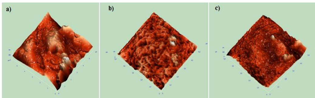
Fig. 2. 3D images of PP/Ag<sub>2</sub>S nanocomposite samples: (a) high rate cooling (water) (50 deg/min), (b) slow cooling (2deg/min) and (c) liquid nitrogen cooling (2000 deg/min).
