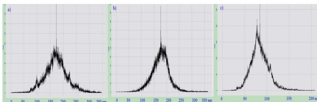
Fig. 3. The surface density distribution (histogram) of nanoparticles in the specific area of the PP/Ag<sub>2</sub>S nanocomposites samples depending on the CTTmode: (a) high rate cooling (water) (50 deg/min), (b) slow cooling (2deg/min) and (c) liquid nitrogen cooling (2000 deg/min).
