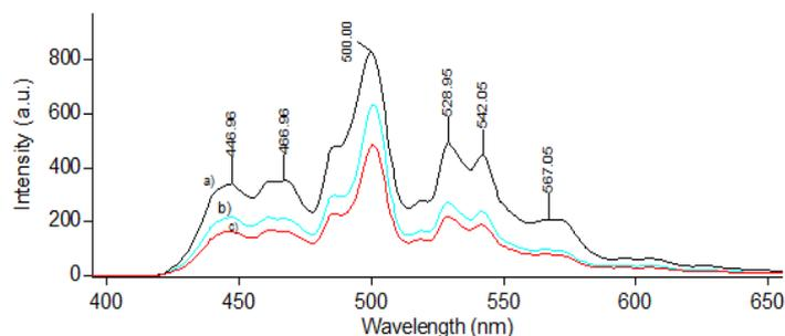
Fig. 5. Luminescence spectra of PP/Ag<sub>2</sub>S nanocomposites obtained in different CTT modes: (a) liquid nitrogen cooling (2000 deg/min), (b) high rate cooling (water) (50 deg/min) and (c) slow cooling (2deg/min)
