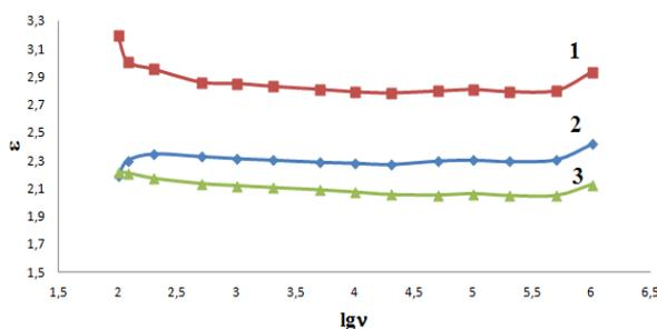
Fig. 6. The frequency dependence graphs of dielectric permeability of the PNC obtained at different CTT modes : (a) slow cooling (2deg/min), (b) liquid nitrogen cooling (2000 deg/min), (c) high rate cooling (water) (50 deg/min).
