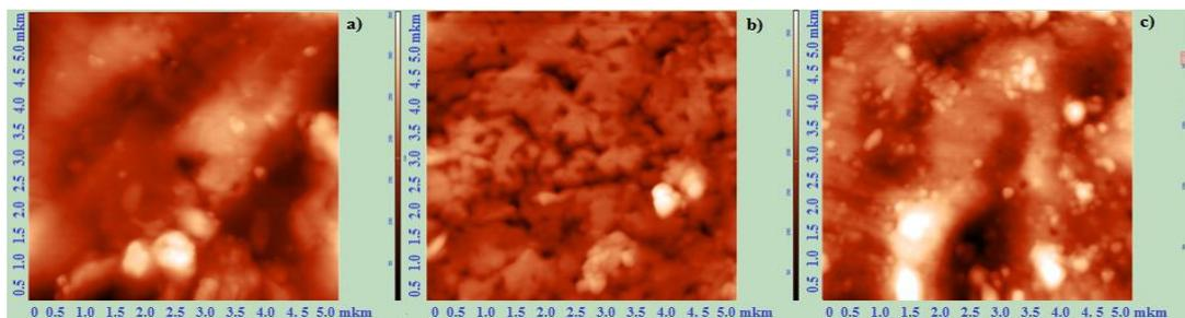
Fig. 1. 2D images of PP/Ag<sub>2</sub>S nanocomposites samples: (a) high rate cooling (water) (50 deg/min), (b) slow cooling (2deg/min) and (c) liquid nitrogen cooling (2000 deg/min).
