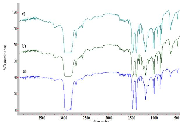
Fig. 4. IR spectra of PP/Ag<sub>2</sub>S nanocomposites at different CTT modes: a) high rate cooling (water) (50 deg/min), b) slow cooling (2deg/min) and c) liquid nitrogen cooling (2000 deg/min).
