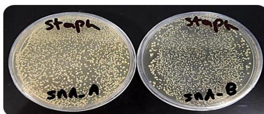
Fig. 12. Antibacterial Test on *Staphylococcus* in Thin Film of a) SnS before Plasma Treatment, and b) SnS after Plasma Treatment
