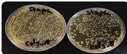
Fig. 14. Antibacterial Test on Staphylococcus in Thin Film of a) CdS before Plasma Treatment, and b) CdS after Plasma Treatment
