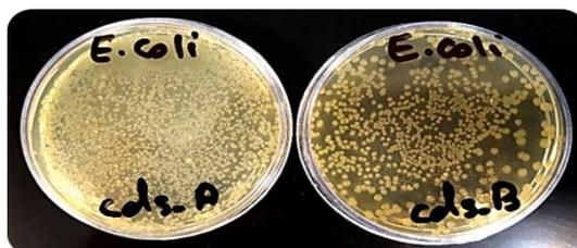
Fig. 15. Antibacterial Test on E.coli in Thin Film of a) CdS before Plasma Treatment, and b) CdS after Plasma Treatment.
