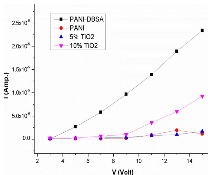
Fig. 3. I-V plot of PANI-EB, PANI-DBSA and PANI/TiO<sub>2</sub>.
