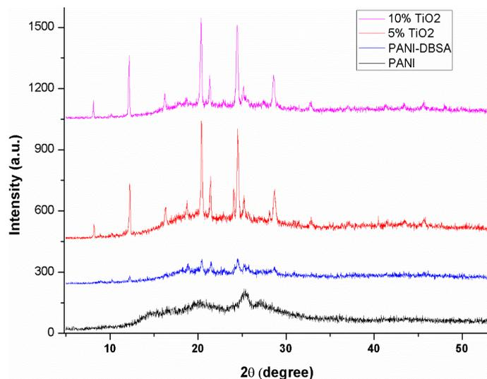
Fig. 2. The recorded XRD peaks of PANI-EB, PANI-DBSA and PANI/TiO<sub>2</sub>.
