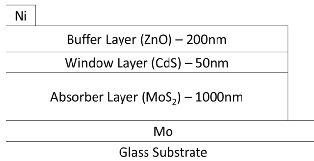
Fig. 1(a): Basic structure of the MoS 2 hetero-junction solar cells
