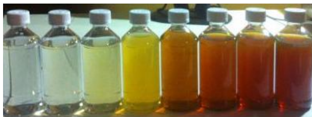
Fig. 2. Color variations depending reduction time of chitosan-Ag 0 suspension
