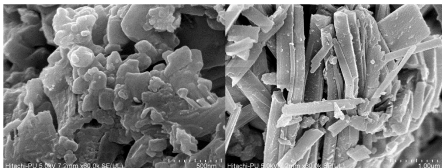
Fig. 10. SEM micrographs of CoS nanoparticles.
