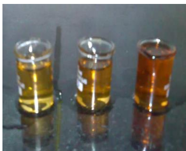
Fig. 1. Colloidal suspension of CdSe QD'S of increasing size at frequent time intervals (2mins, 4mins and 6mins).
