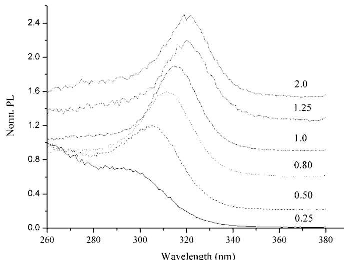
Fig. 4 Excitation PL spectra of ZnS dispersions at various  $S^{2-}/Zn^{2+}$  ratios
