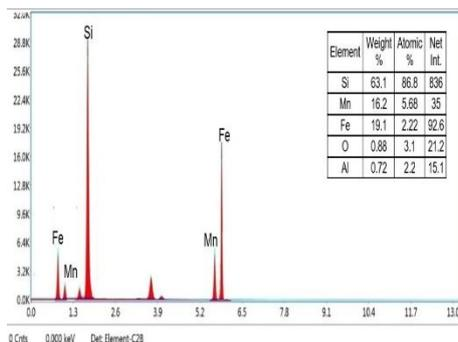
Fig. 5. b) EDX spectrum of  $MnFe_2O_4$  Coated A3 Layer on Silicon solar cell.
