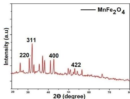
Fig. 2. XRD of Synthesized  $MnFe_2O_4$ .
