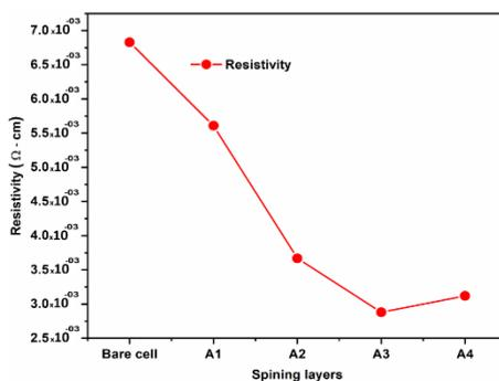
Fig. 7. Resistivity of  $MnFe_2O_4$  samples.
