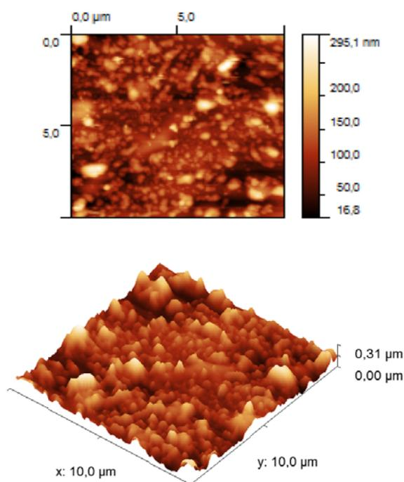
FIG 8. AFM micrography for BiTe films deposited using the ChCl-MA ionic liquid containing 2.5 mM Bi + 2.5 mM Te, at constant potential of -0.35V for 1 hour; temperature 50°C.
