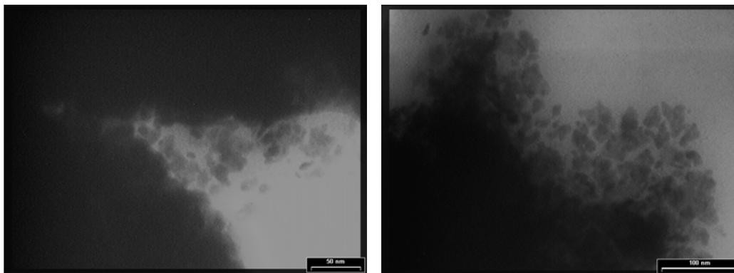
FIG 10. TEM images for BiTe films deposited using the ChCl-MA ionic liquid containing 2.5 mM Bi + 2.5 mM Te, at constant potential of -0.35V for 1 hour; temperature 50°C.
