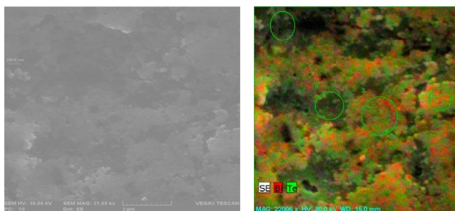
FIG 9. The SEM image (A) and mapping image of elements (B) for BiTe films deposited on copper substrate using the ChCl-MA ionic liquid with 2.5 mM Bi + 2.5 mM Te, at constant potential of -0.35V, 1 hour; temperature 50°C.
