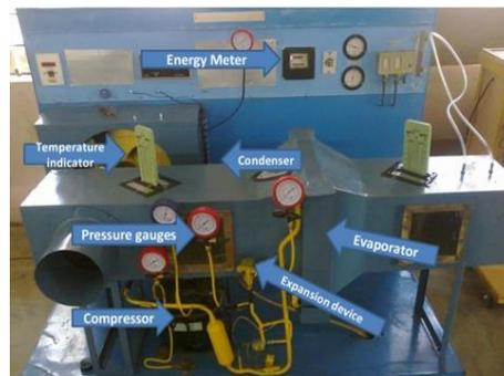
Fig. 10. Schematic representation of Experimental setup.
