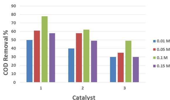
Fig. 7. The COD removal efficiency of BPA as a function of supporting electrolyte concentration (treatment time: 60 min, current density of 15 mA/cm<sup>2</sup>).
