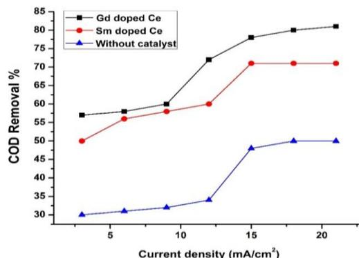
Fig. 8. The COD removal efficiency of resorcinol as a function of applied current density
