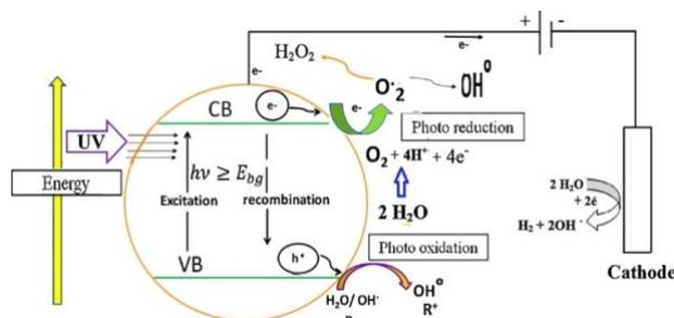
*Scheme. 1 Photo-Electrochemical Reactor*
