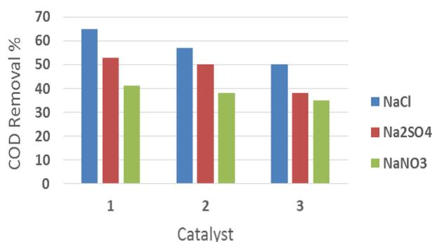
Fig. 5. The COD removal efficiency of BPA as a function of supporting electrolyte
