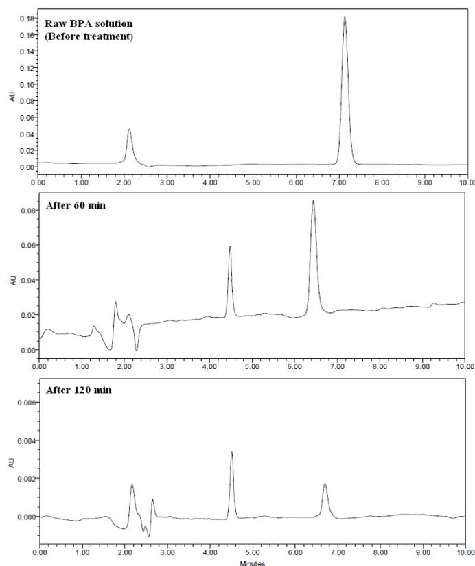
Fig. 11. HPLC analysis of before and after PECO treatment
