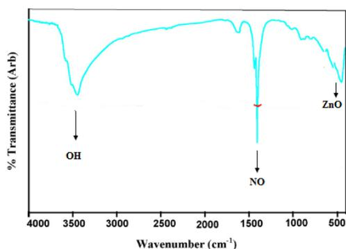
Fig. 3. FTIR spectra of ZnO nano material
