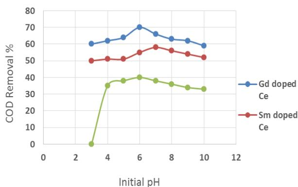
Fig. 6. The COD removal efficiency of BPA as a function of initial pH (treatment time: 60 min, current density of 15mA/cm<sup>2</sup> and distance between electrodes: 7 mm, supporting electrolyte: NaCl 0.1 M).
