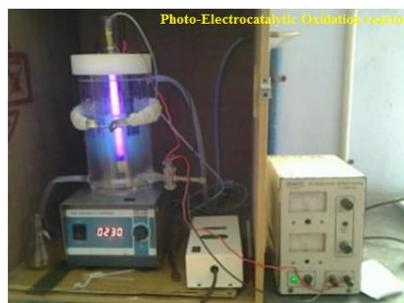
*Fig.1. Experimental setup for photo-electrochemical reactor*
