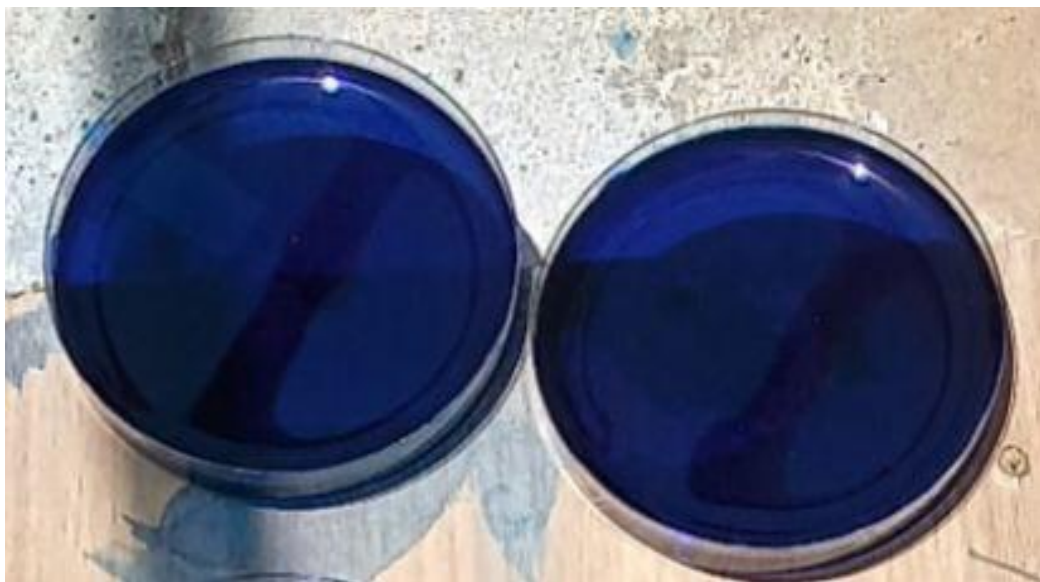
Figure 2. Experimental setup showing the ZnO-Ag 2 O coated substrates immersed in Methylene Blue solution under visible light irradiation.
